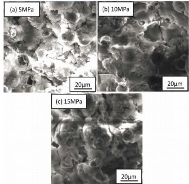
Fig. 2. Microstructure of SiO<sub>2</sub>/Al cermet material prepared by different forming pressure.
