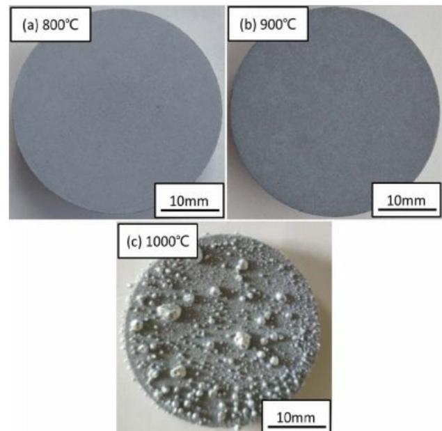
**Fig. 4.** Effect of sintering temperature on surface macroscopic morphology of SiO<sub>2</sub>/Al cermet.
