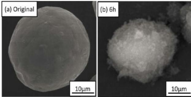
Fig. 1. Microstructure of Al and SiO<sub>2</sub>/Al composite powder.
