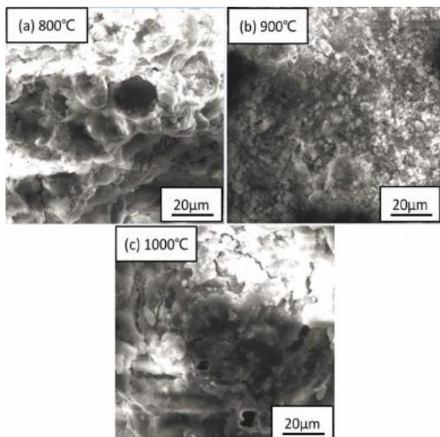
**Fig. 3.** Effect of sintering temperature on microstructure of SiO<sub>2</sub>/Al cermet.
