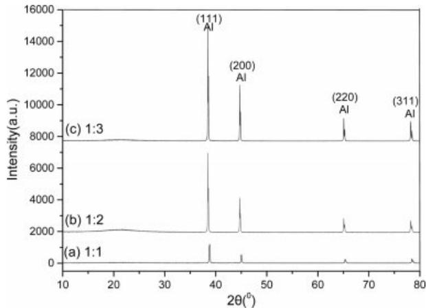
Fig. 5. XRD of samples prepared by different raw materials.
