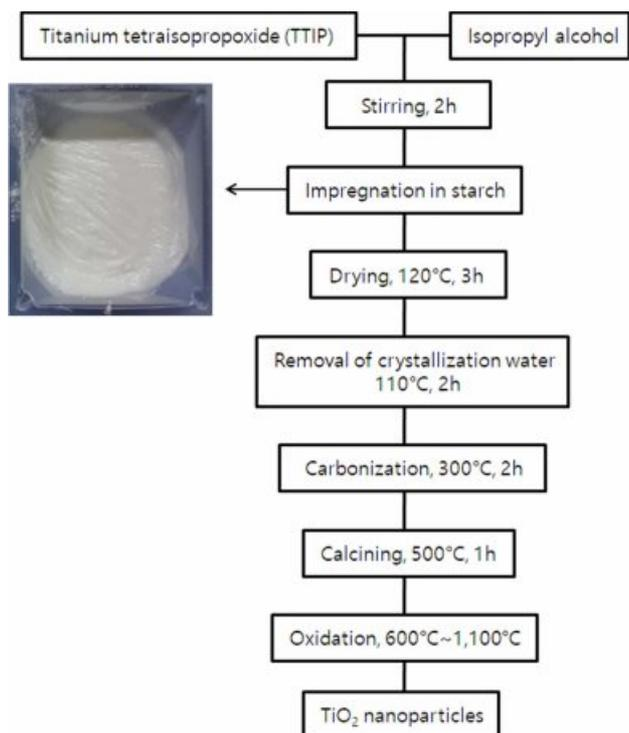
Fig. 1. Preparation procedures of  $\text{TiO}_2$  nano powders.
