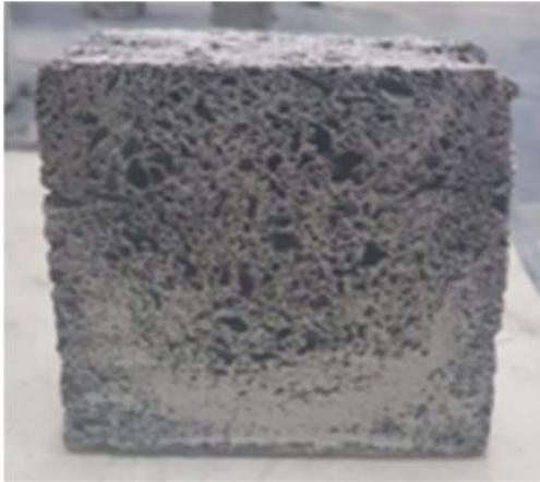
**Fig. 9.** Cross-sectional image of the large ( $400 \times 100 \times 200 \text{ mm}^3$ ) specimen.
