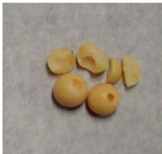
**Fig. 3.** Photograph of  $(\text{Sr}_{0.97}\text{Eu}_{0.03})_4\text{ScAl}_3\text{O}_{10}$  phosphor under the fluorescent lamp.
