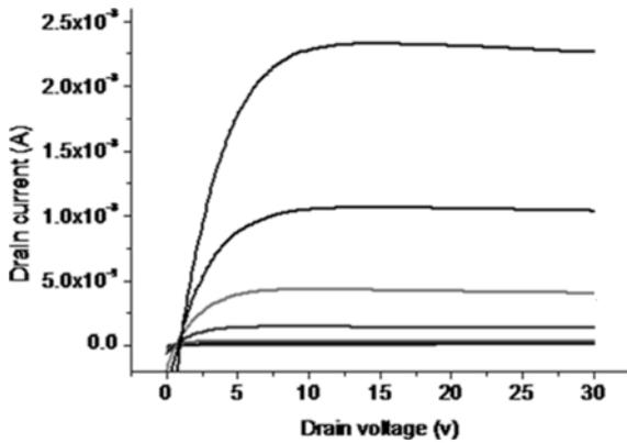
Fig. 5. Output characteristics of a TFT.
