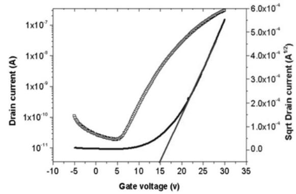
Fig. 6. Input characteristics of a TFT.
