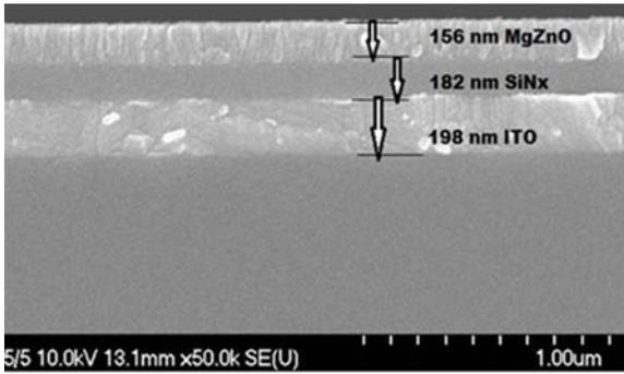
Fig. 4. SEM image of cross section view of the device.
