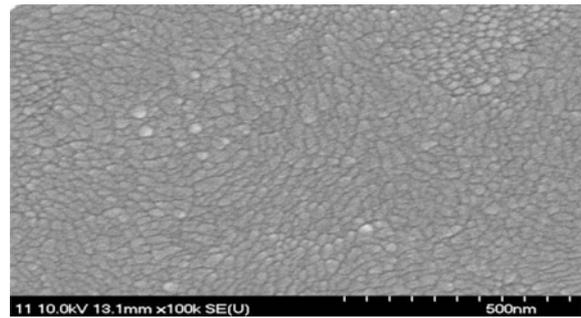
Fig. 1. Surface morphology of MgZnO film grown at 100 °C.
