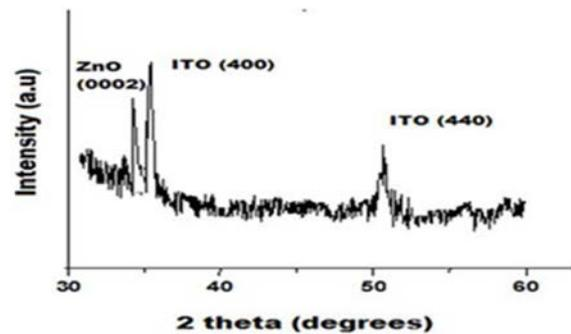
Fig. 2. XRD analysis of MgZnO film grown at 100°C.
