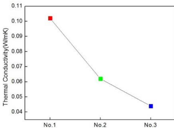
Fig. 6. Thermal conductivity of mineral hydrate insulation.
