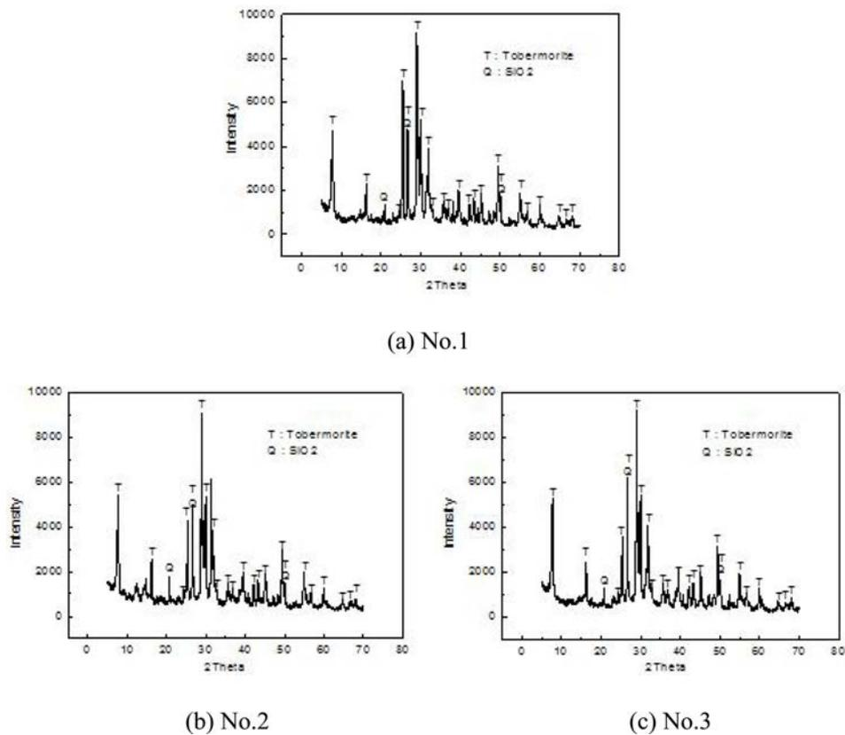
Fig. 4. Properties of crystal of mineral hydrate insulation.
