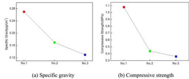
Fig. 2. Physical properties of mineral hydrate insulation in accordance with the fineness of activated cement.
