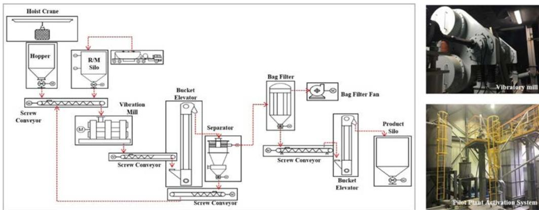
Fig. 1. Pilot plant activation system.
