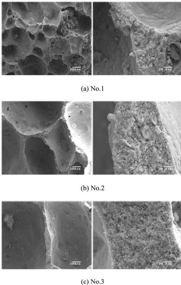
Fig. 5. Microstructure of mineral hydrate insulation.
