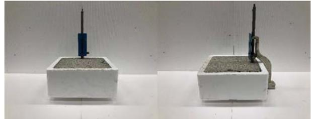
**Fig. 1.** Measurement of hardening time used Vicat apparatus.
