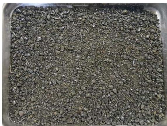
Fig. 2. As-received IGCC slag.
