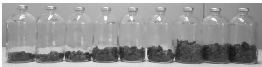
Fig. 6. Photographs of specimens three days after removing medium. The first three bottles from the left: culture on 100 ml medium and 20 g aggregates with 0.5 g/l bacteria, the next three bottles: culture on 100 ml medium and 40 g aggregates with 0.5 g/l bacteria, the last three bottles: culture on 100 ml medium and 60 g aggregates with 0.5 g/l bacteria. Each bottle has the same P<sub>CO<sub>2</sub></sub> and culture period.
