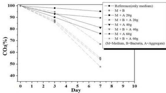
Fig. 4. Results of GC-TCD analyses of the specimens shown in Fig. 3.
