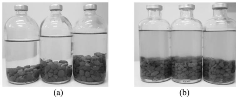
Fig. 5. Photographs of specimen using 27s medium (a) Reference group: 165 ml glass bottles using 100 ml medium and 20, 40, 60 g aggregates (b) Control group: 280 ml glass bottles using 200 ml medium and 120 g aggregates with 0.5 g/l bacteria.
