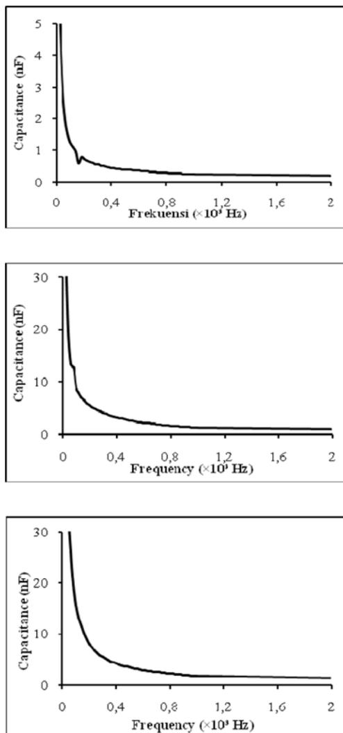
**Fig. 3.** Capacitance of  $\text{CaTiO}_3$  sintered at (A) 700 °C, (B) 800 °C, (C) 900 °C.
