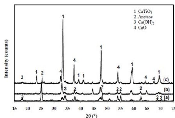
**Fig. 1.** Diffractogram of  $\text{CaTiO}_3$  sample for sintering at (A)  $700^\circ\text{C}$ , (B)  $800^\circ\text{C}$ , dan (C)  $900^\circ\text{C}$ .
