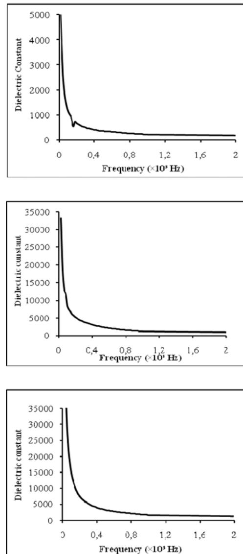
**Fig. 4.** Dielectric constant of  $\text{CaTiO}_3$  sintered at (A) 700 °C, (B) 800 °C, and (C) 900 °C.
