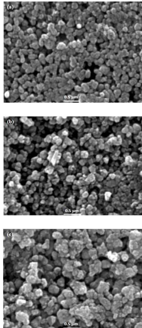
**Fig. 2.** Surface morphology of three TiO<sub>3</sub> sample for sintering at: (A) 700 °C, (B) 800 °C, (C) 900 °C.
