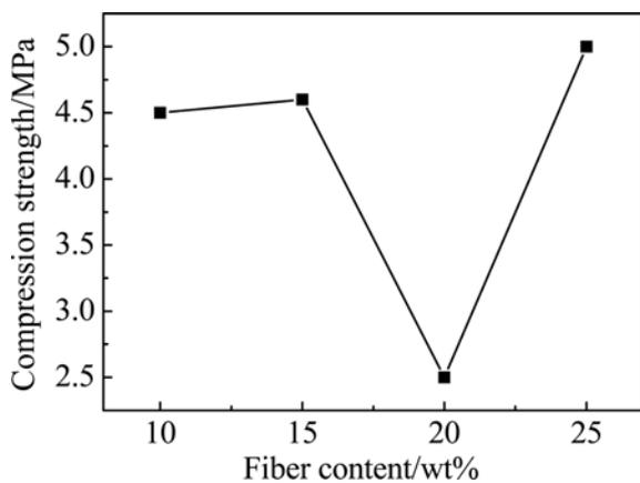
Fig. 6. Effect of the alumina fiber content on the compressive strength of the foam ceramics.
