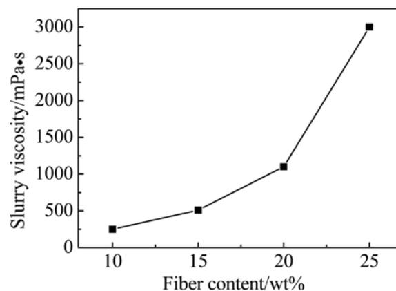
Fig. 1. Effect of the alumina fiber content on the slurry viscosity.
