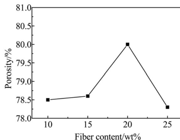
Fig. 2. Effect of the alumina fiber content on the porosity of the prepared ceramics.
