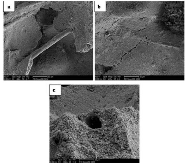
Fig. 4. Microstructure of the sample with the fiber content of 20 wt%.
