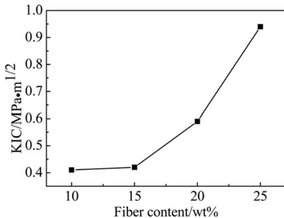
Fig. 5. Effect of the alumina fiber content on the toughness of the foam ceramics.
