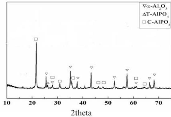
Fig. 3. XRD pattern of the sintered sample.
