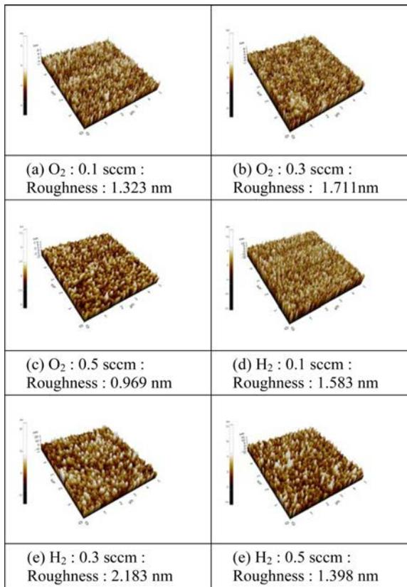
Fig. 3. AFM morphologies of the MZO films deposited with different ambient gases.
