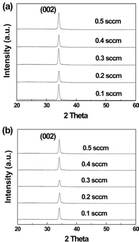
**Fig. 1.** XRD patterns of MZO thin films deposited under (a) O<sub>2</sub> and (b) H<sub>2</sub> with Ar gas.
