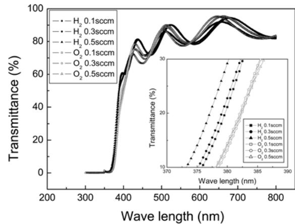
Fig. 5. Optical transmittance spectra of MZO films deposited under different ambient gases (Ar, Ar+ $O_2$ , and Ar+ $H_2$ ).
