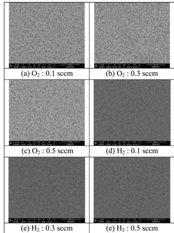
**Fig. 2.** FESEM images of MZO thin films with different ambient gases.<sup>1</sup>
