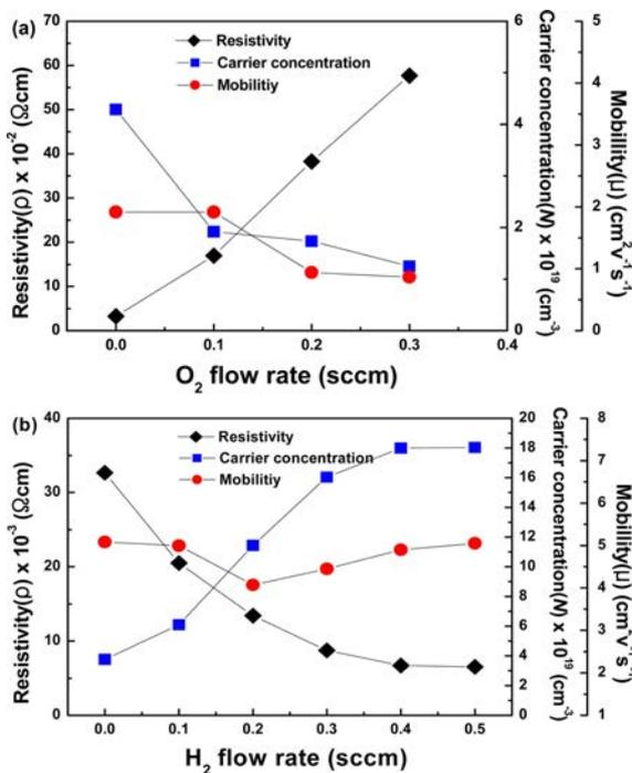
Fig. 4. Resistivity ( $\rho$ ), mobility ( $\mu$ ) and carrier concentration ( $N$ ) of MZO thin films with flow rate of (a)  $O_2$  and (b)  $H_2$  with Ar.
