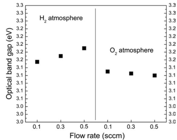
Fig. 6. Optical band gap of MZO thin films as a function of the flow rate of  $O_2$  and  $H_2$  with Ar.
