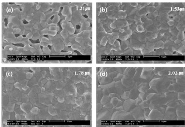
**Fig. 2.** FE-SEM surface image of  $\text{Ni}_{0.79}\text{Mn}_{2.21-x}\text{Cu}_x\text{O}_4$  thick film with variation of Cu content: (a)  $x = 0$  (b)  $x = 0.05$  (c)  $x = 0.10$  (d)  $x = 0.15$ .
