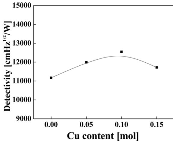
Fig. 6. Detectivity of  $\text{Ni}_{0.79}\text{Mn}_{2.21-x}\text{Cu}_x\text{O}_4$  thick film with variation of Cu content: (a)  $x = 0$  (b)  $x = 0.05$  (c)  $x = 0.10$  (d)  $x = 0.15$ .
