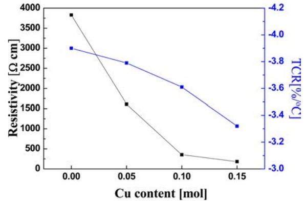
**Fig. 4.** Resistivity at room temperature and TCR of  $\text{Ni}_{0.79}\text{Mn}_{2.21-x}\text{Cu}_x\text{O}_4$  thick film with variation of Cu content: (a)  $x = 0$  (b)  $x = 0.05$  (c)  $x = 0.10$  (d)  $x = 0.15$ .
