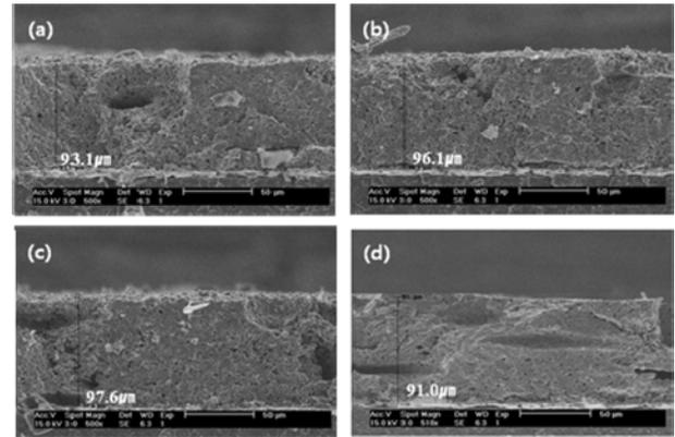
**Fig. 3.** FE-SEM Cross-section image of  $\text{Ni}_{0.79}\text{Mn}_{2.21-x}\text{Cu}_x\text{O}_4$  thick film with variation of Cu content: (a)  $x = 0$  (b)  $x = 0.05$  (c)  $x = 0.10$  (d)  $x = 0.15$ .
