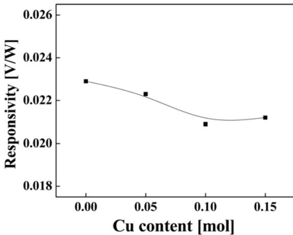
Fig. 5. Responsivity of  $\text{Ni}_{0.79}\text{Mn}_{2.21-x}\text{Cu}_x\text{O}_4$  thick film with variation of Cu content: (a)  $x = 0$  (b)  $x = 0.05$  (c)  $x = 0.10$  (d)  $x = 0.15$ .
