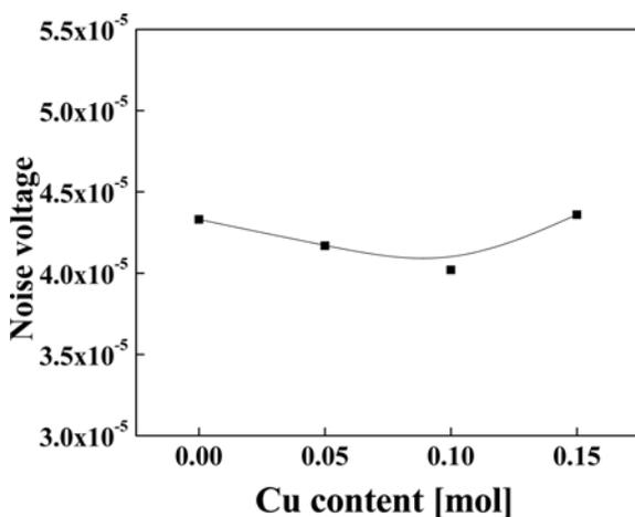
Fig. 7. Voltage noise of  $\text{Ni}_{0.79}\text{Mn}_{2.21-x}\text{Cu}_x\text{O}_4$  thick film with variation of Cu content: (a)  $x = 0$  (b)  $x = 0.05$  (c)  $x = 0.1$  (d)  $x = 0.15$ .
