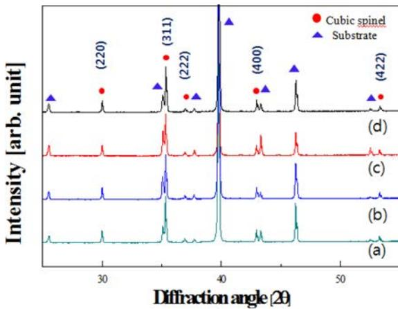
**Fig. 1.** X-Ray Diffraction pattern of  $\text{Ni}_{0.79}\text{Mn}_{2.21-x}\text{Cu}_x\text{O}_4$  thick film with variation of Cu content: (a)  $x = 0$  (b)  $x = 0.05$  (c)  $x = 0.10$  (d)  $x = 0.15$ .
