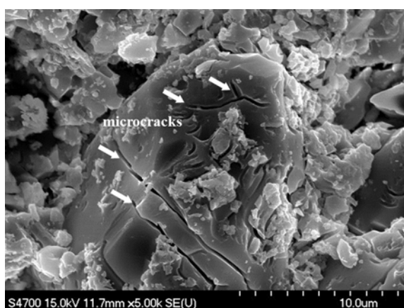
Fig. 3. Microcracks on fused silica by phase transformation.
