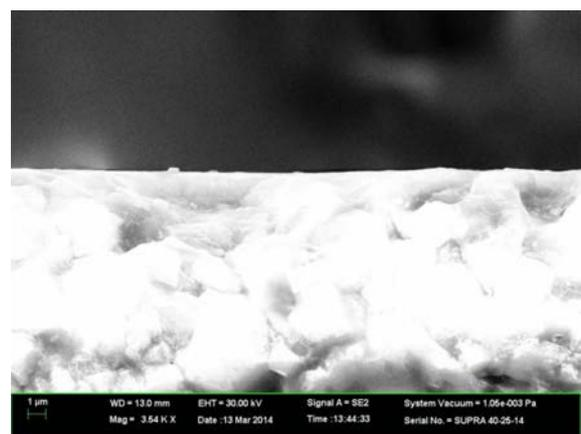
**Fig. 3.** Cross-sectional FE-SEM of the UNSM-treated specimen showing a modified layer in the topmost surface layer.
