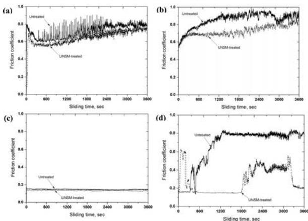
**Fig. 4.** Variations in friction coefficient as a function of reciprocating sliding time of the untreated and UNSM-treated  $\text{Al}_2\text{O}_3$  specimens under dry (a, b) and oil-lubricated (c, d) conditions at temperatures of 25 and 200 °C, respectively.
