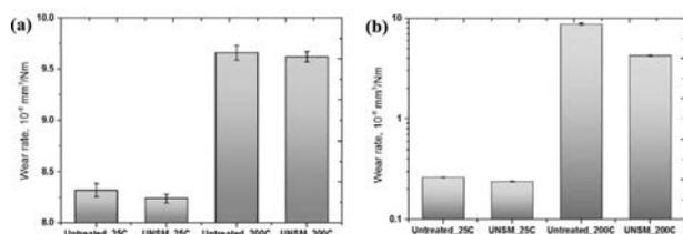
**Fig. 7.** Wear rate of the untreated and UNSM-treated  $\text{Al}_2\text{O}_3$  specimens under dry and oil-lubricated conditions at temperatures of 25 and 200 °C, respectively.
