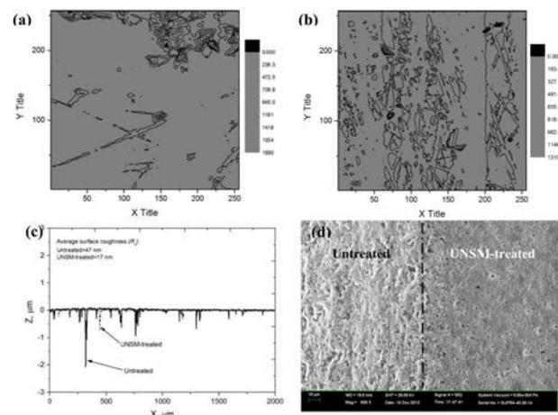
**Fig. 1.** Comparison of surface morphology (a, b), surface roughness profile (c) and microstructure (d) of the untreated and UNSM-treated  $\text{Al}_2\text{O}_3$  specimens. 2D AFM scan area of  $100\ \mu\text{m} \times 100\ \mu\text{m}$ .
