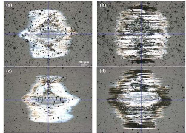
**Fig. 5.** LSM images of wear tracks of the untreated (a, b) and UNSM-treated (c, d)  $\text{Al}_2\text{O}_3$  specimens under dry conditions at temperature of 25 and 200 °C, respectively.
