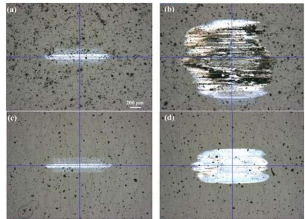
**Fig. 6.** LSM images of wear track of the untreated (a, b) and UNSM-treated (c, d)  $\text{Al}_2\text{O}_3$  specimens under oil-lubricated conditions at temperature of 25 and 200 °C, respectively.
