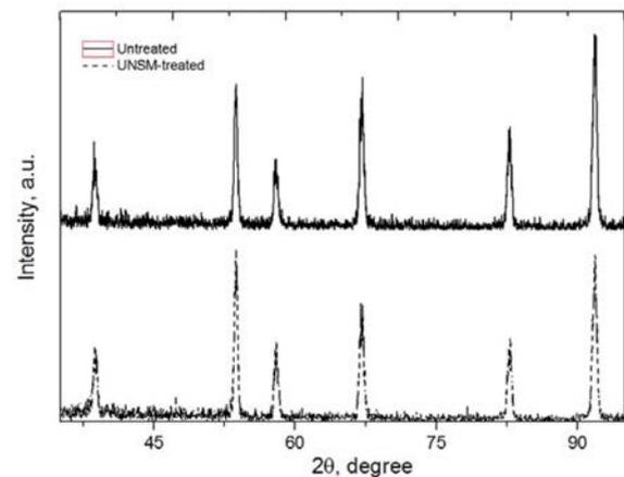
**Fig. 2.** X-ray diffraction patterns of the untreated and UNSM-treated specimens.
