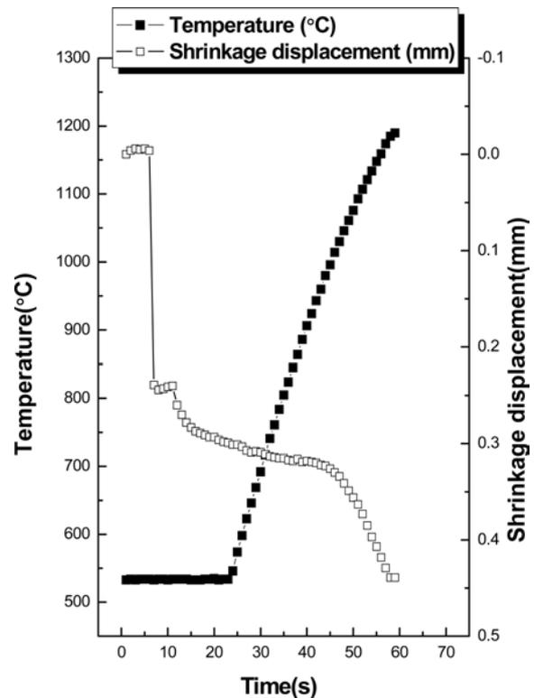
**Fig. 5.** Variation in temperature and shrinkage displacement with heating time during high frequency induction heated sintering of TiCo- $\text{Al}_2\text{O}_3$  systems.
