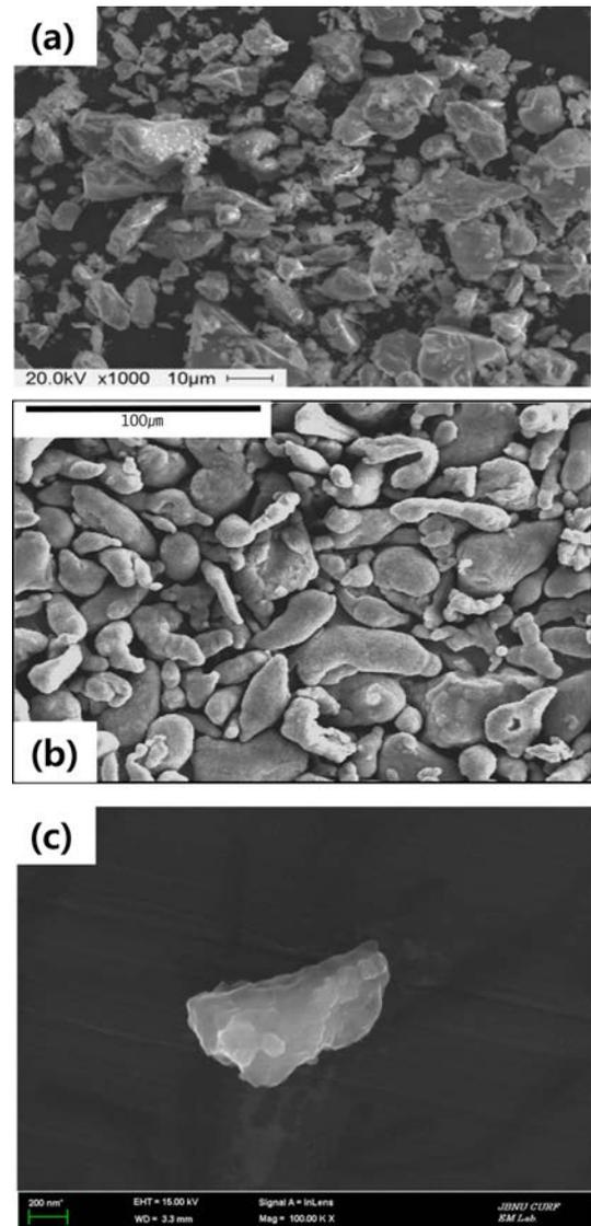
**Fig. 2.** FE-SEM images of (a) CoTi<sub>3</sub>, (b) Al and (c) mechanically synthesized powder.
