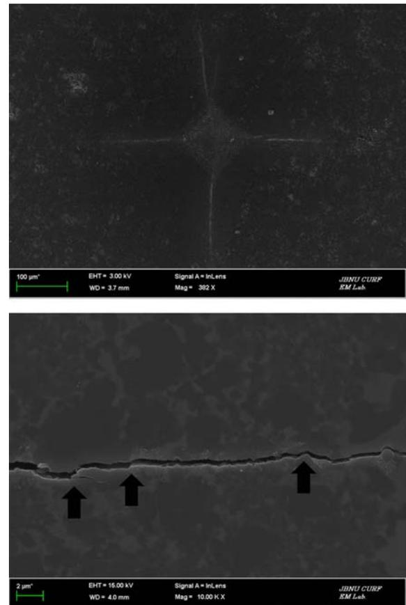
**Fig. 8.** (a) Vickers hardness indentation and (b) median crack propagation in the TiCo-Al<sub>2</sub>O<sub>3</sub> composite.
