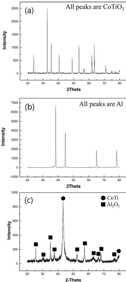
**Fig. 3.** XRD patterns of (a)  $\text{CoTi}_3$ , (b) Al and (c) mechanically synthesized powder.
