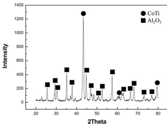
**Fig. 7.** X-ray diffraction pattern of TiCo-Al<sub>2</sub>O<sub>3</sub> composite sintered at 1200 °C.
