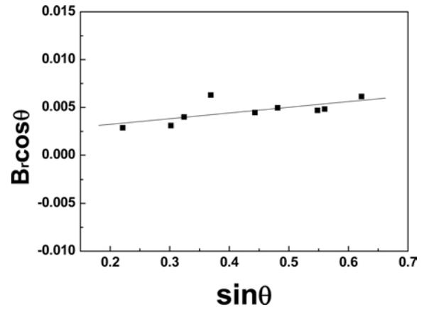
**Fig. 4.** Plot of  $\sin\theta$  versus  $B_r\cos\theta$  for  $\text{Al}_2\text{O}_3$  in mechanically milled powder.
