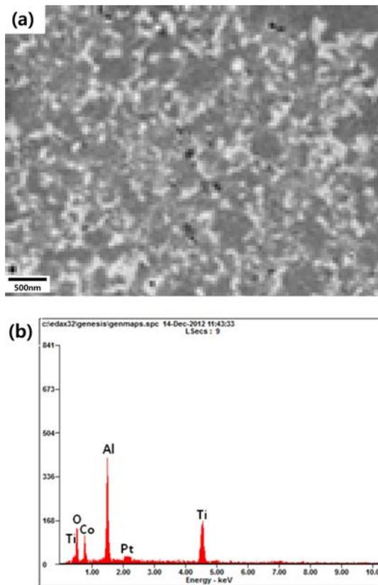
**Fig. 6.** (a) FE-SEM image and (b) EDS of TiCo-Al<sub>2</sub>O<sub>3</sub> composite heated to 1200 °C.
