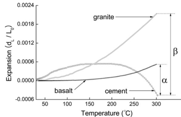
Fig. 2. Thermal expansion of aggregates, relative to cement paste.
