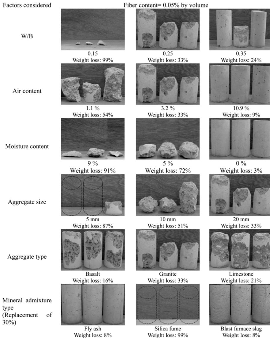
**Fig. 1.** Photo & weight loss of specimens after fire exposure.
