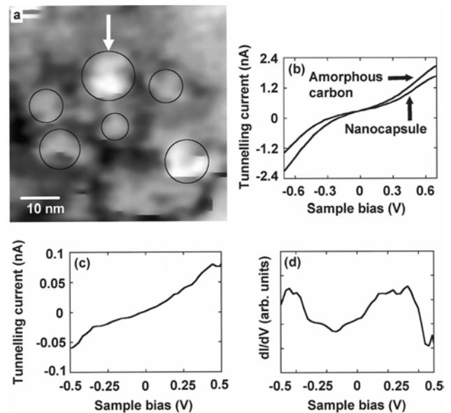
**Fig. 2.** (a) STM image of carbon nanocapsules with gold nanoparticles on the a-C thin film. (b) I-V curves of background and the single C nanocapsule indicated by an arrow in Fig. 2(a). (c) I-V curve of the single C nanocapsule, calculated by subtracting background data from whole data in Fig. 2(b). (d) Conductivity curve of the carbon nanocapsule calculated from the I-V curve in Fig. 2(c).
