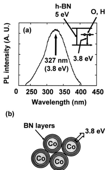
**Fig. 5.** (a) PL spectrum of BN nanocapsules with Co nanoparticles. (b) Schematic illustration of PL of BN nanocapsules.
