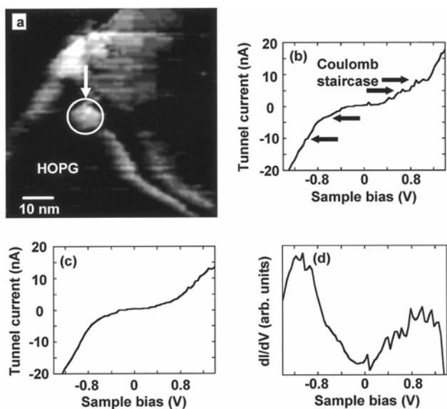
**Fig. 4.** (a) STM image of the BN nanocapsule with the Co nanoparticle on HOPG. (b) I-V characteristic of the single BN nanocapsule, indicated by an arrow in Fig. 4(a). (c) I-V characteristic of HOPG. (d) Conductivity curve of the BN nanocapsule calculated from the I-V curve in Fig. 4(b).
