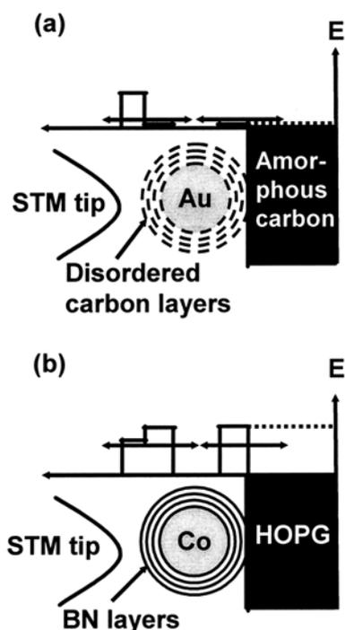
**Fig. 6.** Schematic illustration of the I-V measurements for (a) C nanocapsule and (b) BN nanocapsule.
