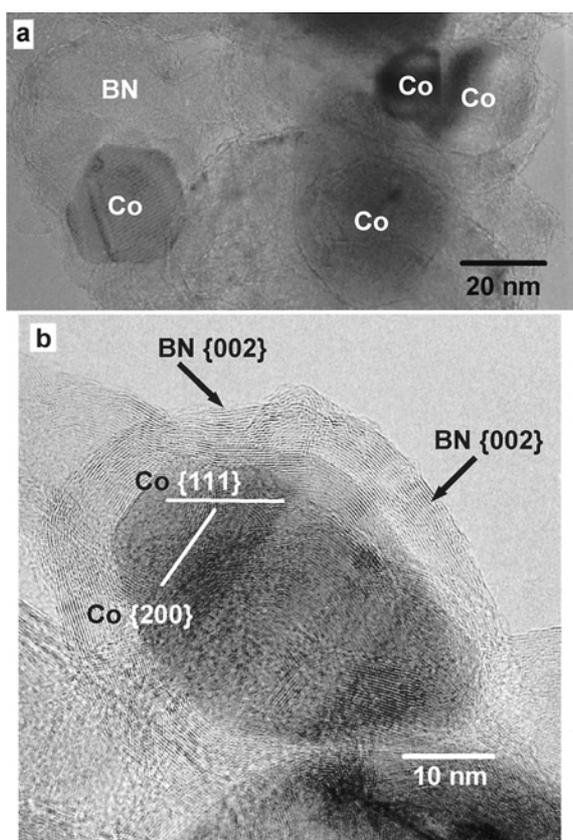
**Fig. 3.** (a) HREM image of BN nanocapsules with cobalt nanoparticles. (b) Enlarged image of a BN nanocapsule with a Co nanoparticle.
