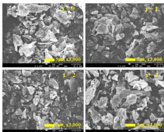
Fig. 3. FE-SEM images of  $\text{BaAl}_2\text{Si}_2\text{O}_8 : \text{Eu}^{2+} + x\text{SiO}_2$  ( $x = 0, 1, 2$  and  $3$ ).
