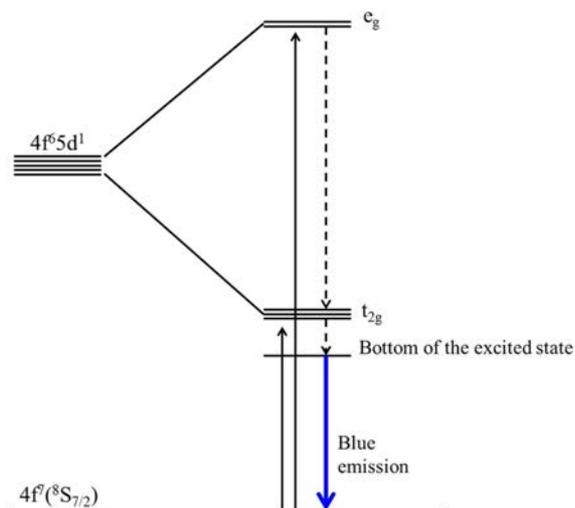
**Fig. 5.** The effect of crystal field splitting on energy level of  $\text{Eu}^{2+}$  in  $\text{BaAl}_2\text{Si}_2\text{O}_8$ .
