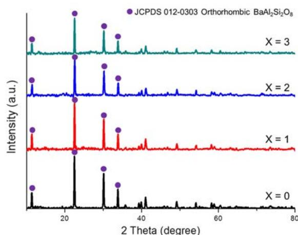
Fig. 2. XRD patterns of  $\text{BaAl}_2\text{Si}_2\text{O}_8 : \text{Eu}^{2+} + x\text{SiO}_2$  ( $x = 0, 1, 2$ , and  $3$ ).
