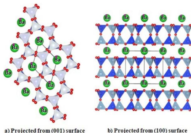
**Fig. 1.** The Crystalline structure of  $\text{BaAl}_2\text{Si}_2\text{O}_8$ .
