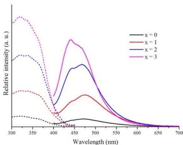
**Fig. 4.** Photoluminescence spectra of  $\text{BaAl}_2\text{Si}_2\text{O}_8 : \text{Eu}^{2+} + x\text{SiO}_2$  ( $x = 0, 1, 2$  and  $3$ ).
