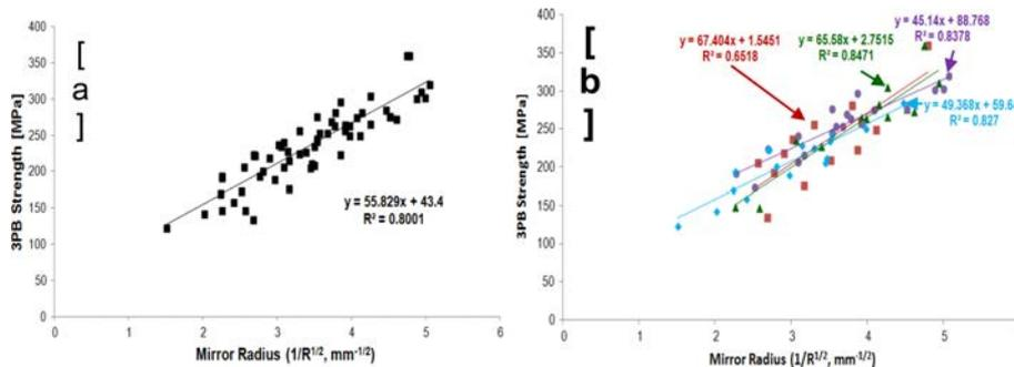
Fig. 4. Plot of the strength data versus the [a] mirror constant calculated with all data points, [b] mirror constant calculated as a function of the span length (60 mm, 80 mm, 100 mm, 120 mm).
