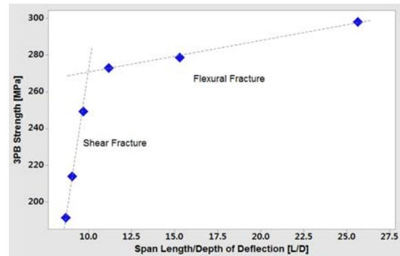
Fig. 1. Bending strength according to the span length/depth of deflection ratio.
