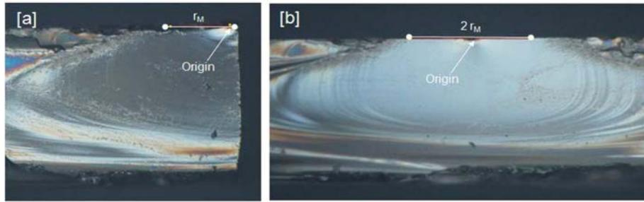
Fig. 2. Fracture surface with a fracture origin and a mirror radius. [a] edge origin, [b] surface origin.
