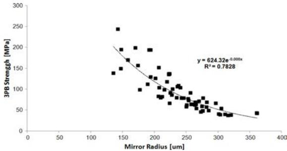
Fig. 3. Plot of the strength data versus the mirror radius; measured with all samples (60 mm, 80 mm, 100 mm, 120 mm).
