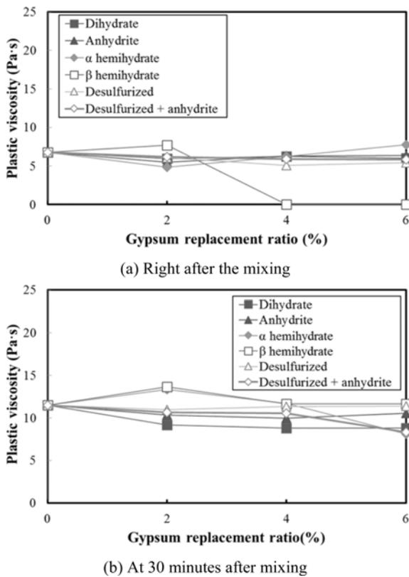
Fig. 9. Influence of various gypsums replacement ratio on plastic viscosity.
