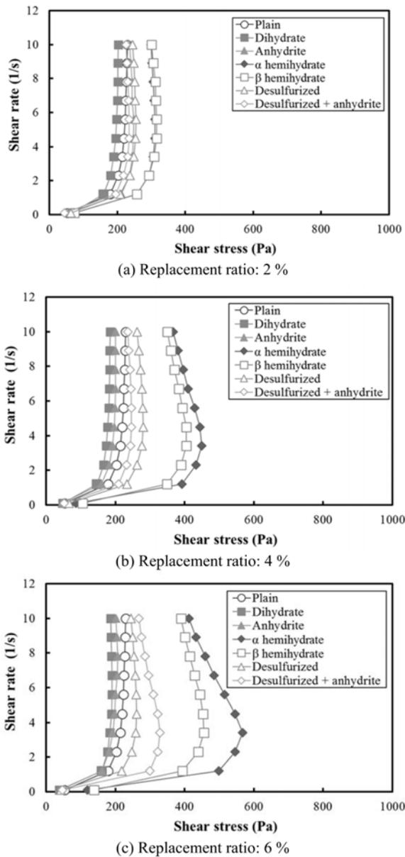
Fig. 7. Influence of various gypsums replacement ratio on flow curves at 30 minutes after mixing.
