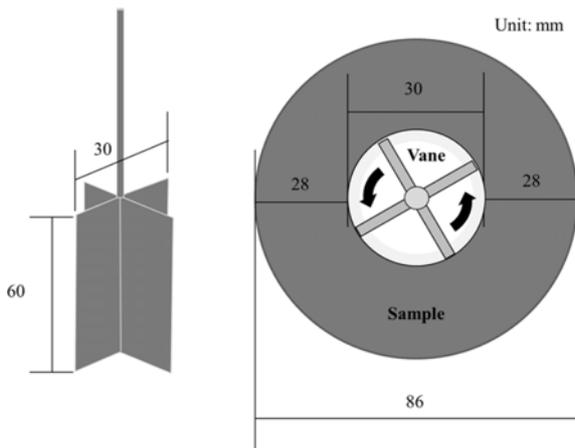
**Fig. 2.** Dimensions of spindle for rheometer.
