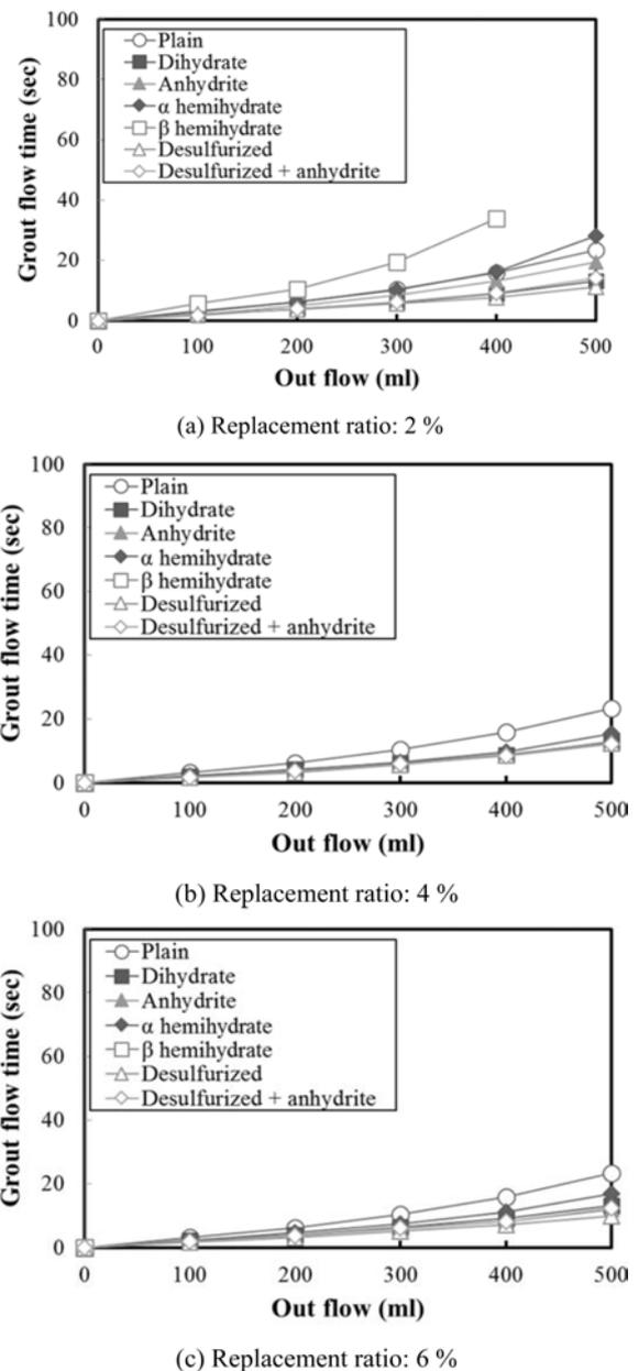
Fig. 4. Influence of various gypsums replacement ratio on grout flow results right after the mixing.
