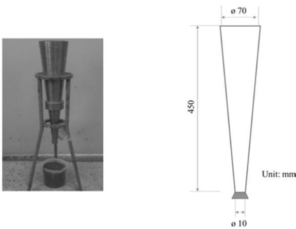
**Fig. 1.** Modified grout flow set up with drawing showing dimensions of the flow funnel.
