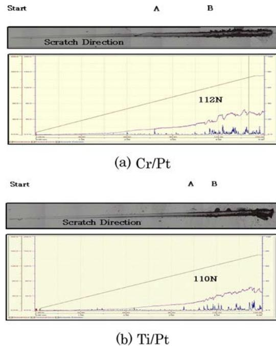
**Fig. 7.** Critical load ( $L_c$ ) and scratch track of Pt thin films on WC substrate measured by scratch test.
