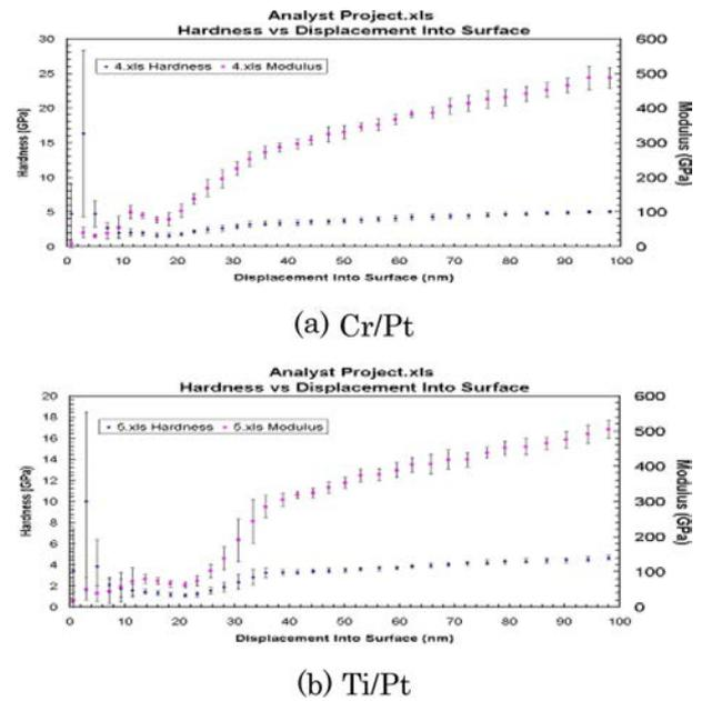
**Fig. 6.** Surface hardness and modulus of (a) Cr/Pt and (b) Ti/Pt thin films on a WC substrate as function of depth.
