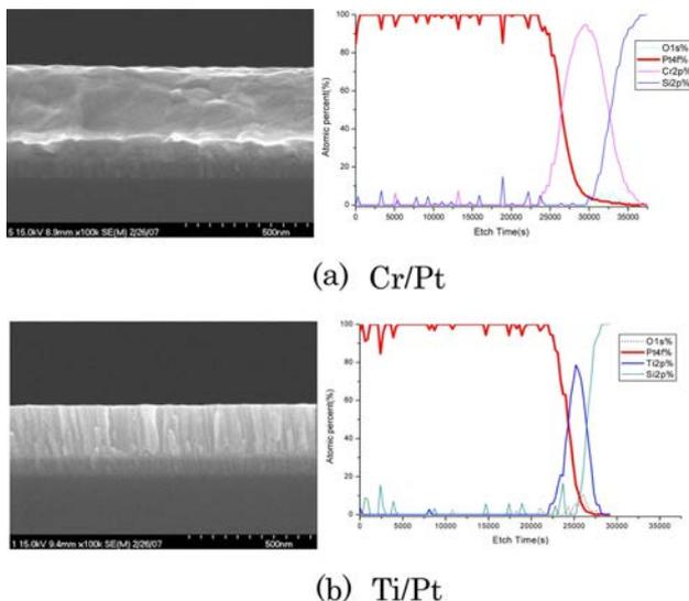
**Fig. 5.** ESCA depth profiles of (a) Cr/Pt and (b) Ti/Pt thin films coated on a Si substrate by ion beam-assisted DC magnetron sputtering.
