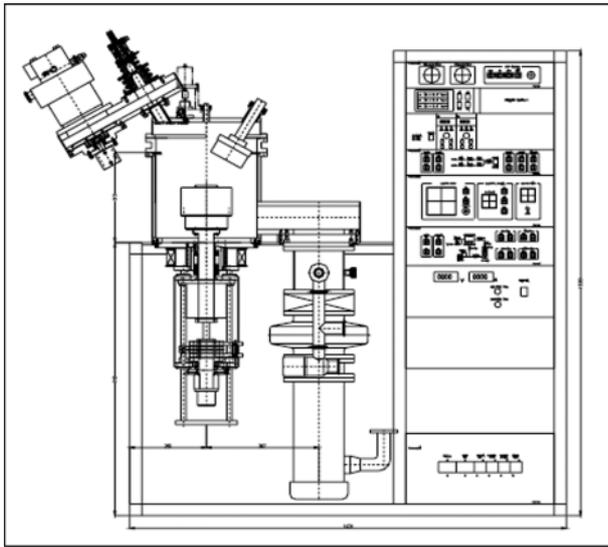
**Fig. 1.** Schematic of an unbalanced DC Magnetron Sputter with Ion Gun.
