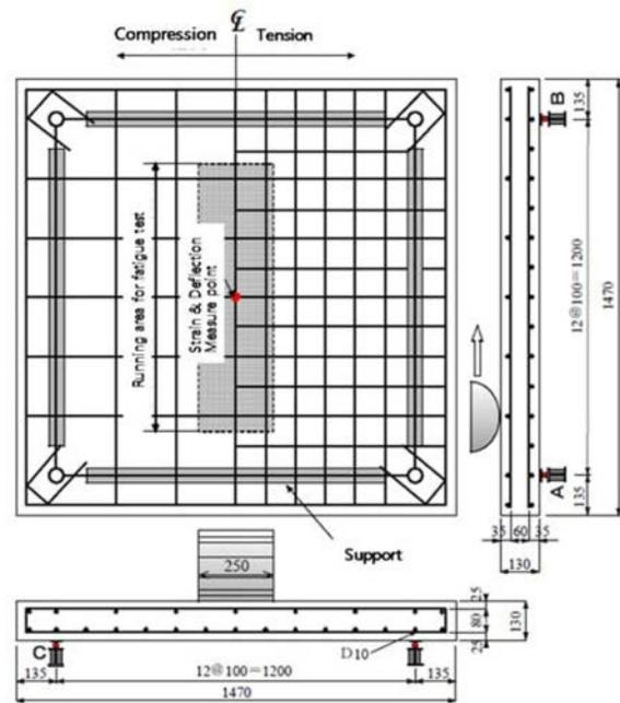
Fig. 5. Specimen size and rebar arrangement.
