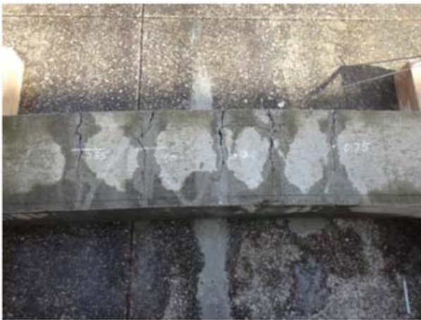
Fig. 5. Crack induction of reinforced concrete.
