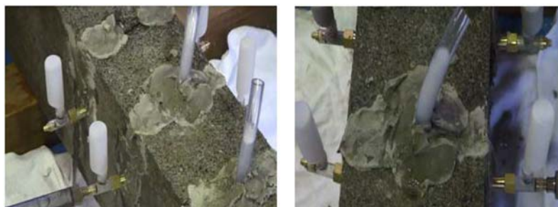
Fig. 8. Injection situation of inorganic water-stop agent.
