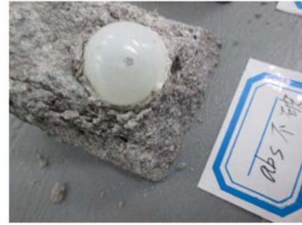
(b) ABS capsule remained intact in a compressed specimen
