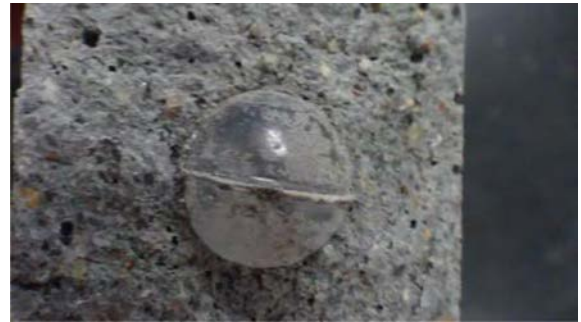
Fig. 14. Morphology of a sheared specimen with an intact capsule.
