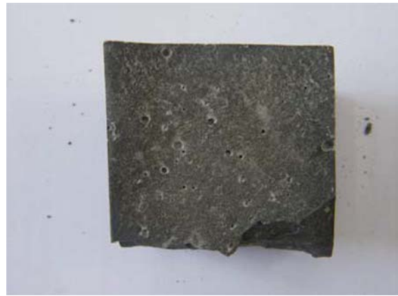
Fig. 2. A specimen of microcapsule based self-healing cementitious materials.
