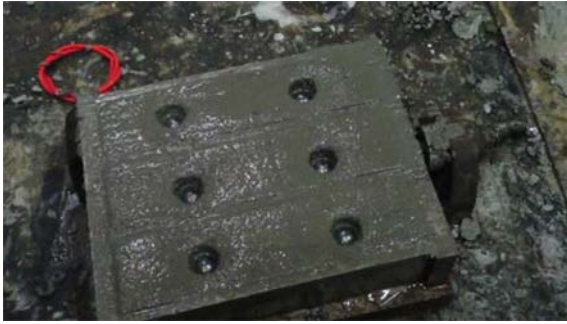
Fig. 10. Specimens with two capsules embedded for shear test.
