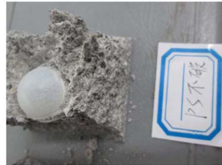
(c) GPPS capsule remained intact in a compressed specimen
