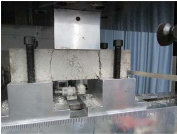
Fig. 11. Shear test of a mortar specimen.
