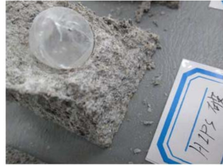
(a) Ruptured HIPS capsule in a compressed specimen
