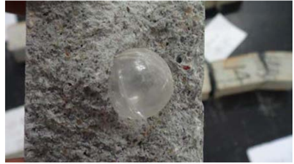
Fig. 13. Morphology of a sheared specimen with a ruptured capsule.
