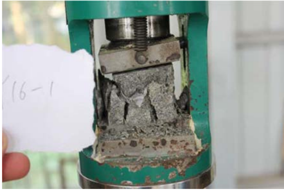
Fig. 7. Compression test of a mortar specimen with a capsule.
