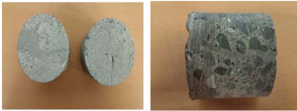
Fig. 6. Core samples from cracked concrete after injection of organic/inorganic composites.
