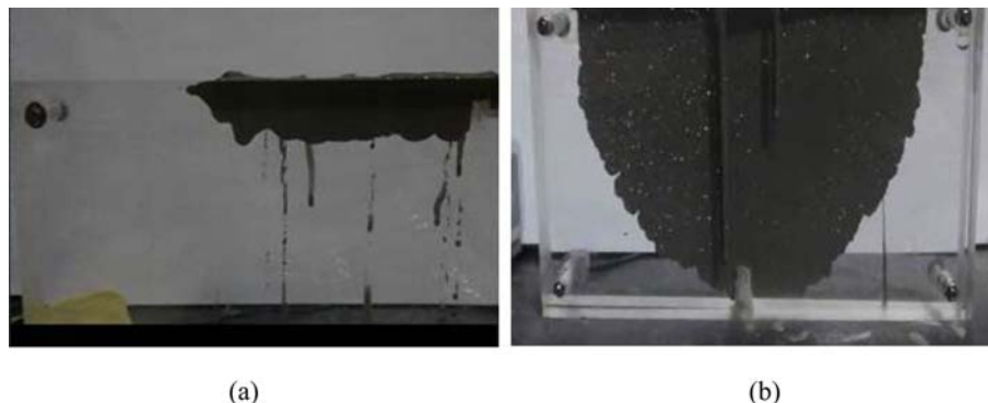
Fig. 5. Injection depth and Shaped test. (a) injection performance of inorganic materials, (b) injection performance of organic and inorganic composite.
