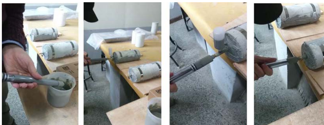
Fig. 7. Injection test of organic and inorganic composite materials on the cracked specimens
