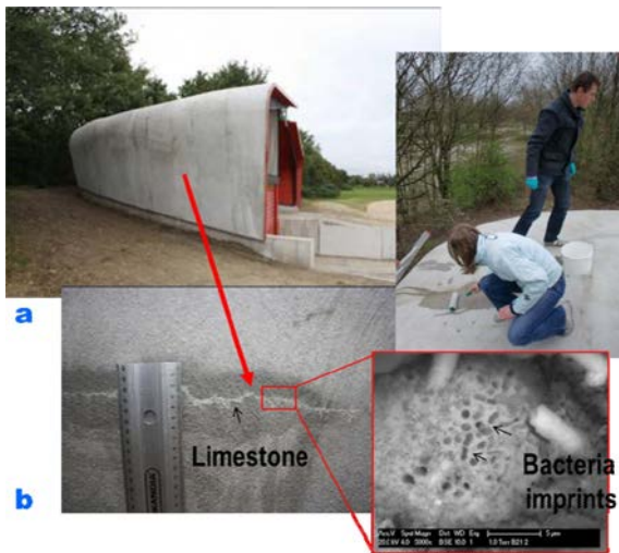
Fig. 8. Cracked concrete structure and crack sealing after impregnating with liquid-based repair system.
