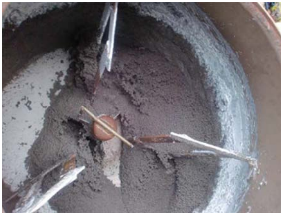
Fig. 1. Impregnation on-site of expanded clays with bacterial spores and organic compound as food for the bacteria.
