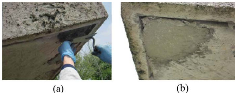
Fig. 4. Self-healing mortar applied under dry conditions: (a) fresh state, (b) after 4 months.
