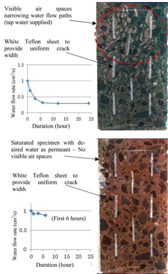
**Fig. 10.** Characteristic effect of air bubble in the initial stage of water supply under unsaturated condition and saturated condition with de-aired & tap water.
