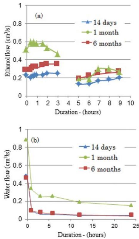
Fig. 7. (a) Ethanol flow rate and (b) water flow rate characteristics through concrete crack.
