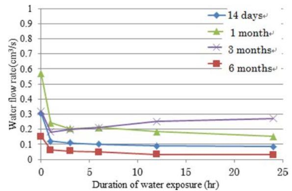
**Fig. 4.** Water flow graph to show possible effect of unhydrated cement content on self-healing.
