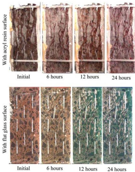
**Fig. 9.** Air bubbles observed through acrylic resin and glass-tap water is used as permeant.
