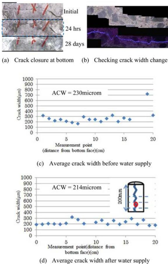
Fig. 6. Checking of crack closing action by measurement of average crack widths before and after water supply in the initial.
