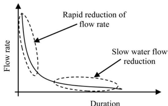
**Fig. 1.** Illustration of general water flow rate Vs duration graph for self-healing tests.
