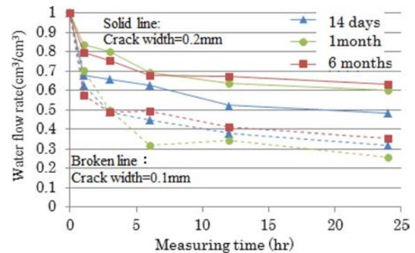
**Fig. 5.** Normalized flow rates to check effect of unhydrated cement on water flow.
