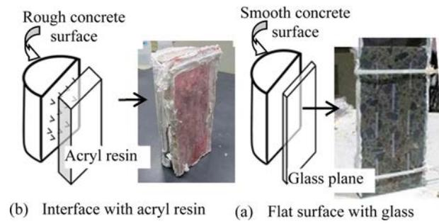
**Fig. 8.** Specimens layout for direct visual observation of water flow through concrete crack.
