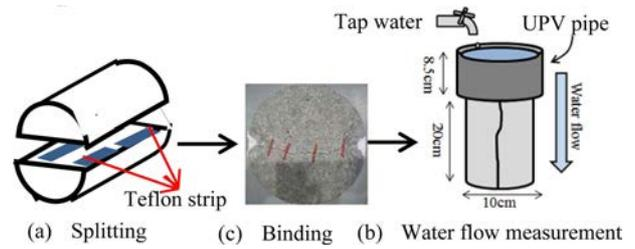
**Fig. 3.** Water flow test measurement procedure.
