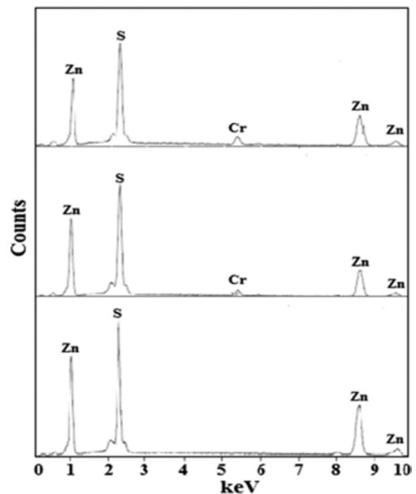
Fig. 3. EDS analysis of pure and Cr doped ZnS nanostructures.
