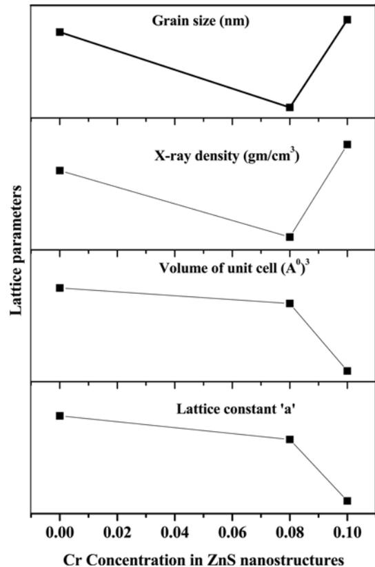
Fig. 2. Variation of lattice parameters with Cr concentration in ZnS nanostructures.
