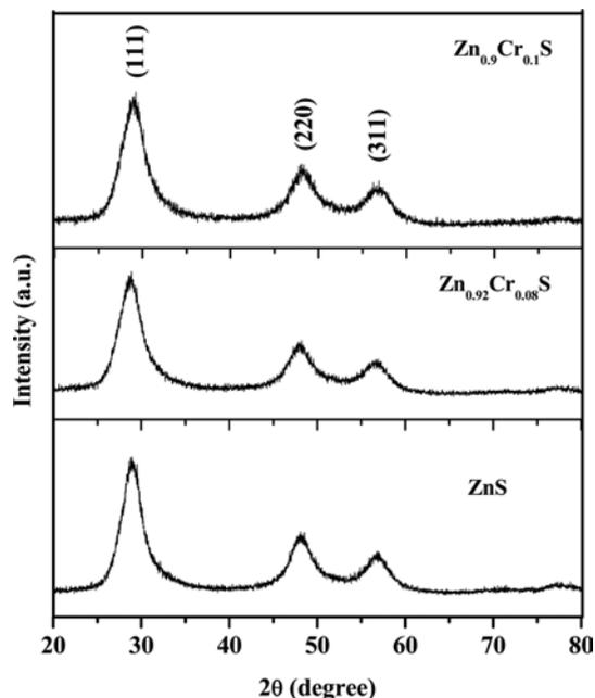
Fig. 1. XRD patterns of pure and Cr doped ZnS nanostructures.
