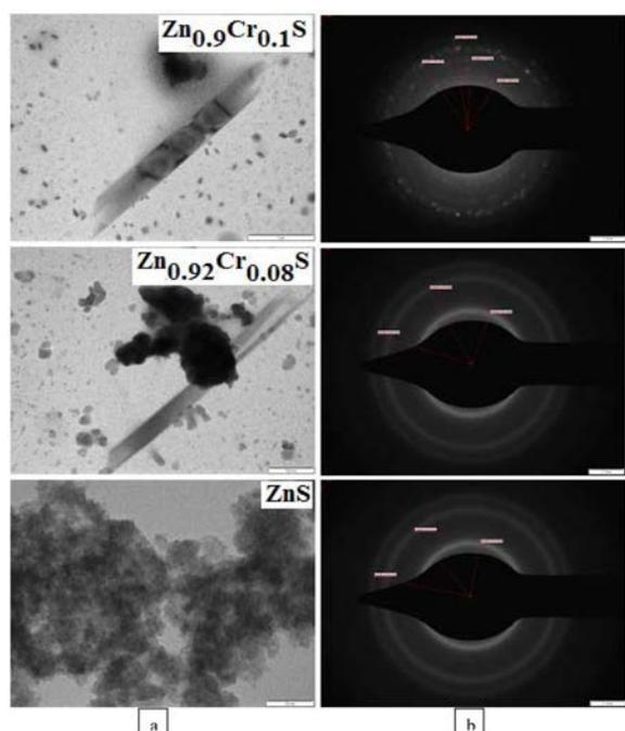
**Fig. 4.** (a) TEM images and (b) SAED pattern of undoped and Cr doped ZnS nanostructures.
