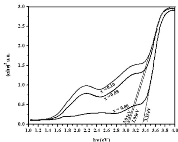
**Fig. 6.** Tauc's plots for pure and Cr doped ZnS nanostructures.
