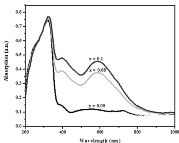
**Fig. 5.** Absorption spectra of pure and Cr doped ZnS nanostructures.
