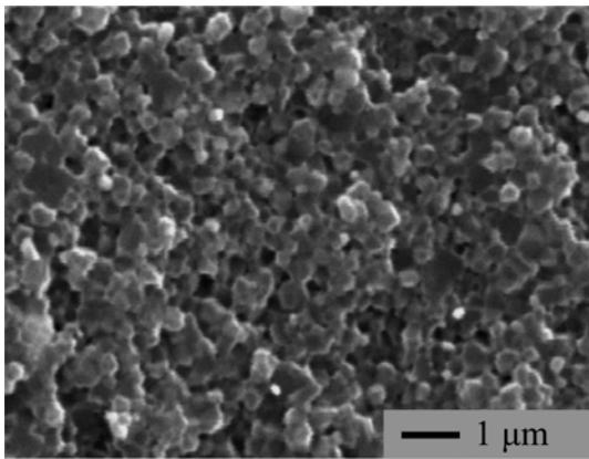
Fig. 1. SEM image shows fractured surface of as-sintered sample.
