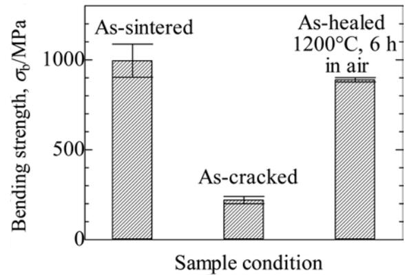
**Fig. 5.** Bending strength of as-sintered, as-cracked and as-healed samples.
