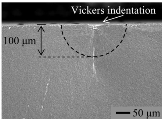
Fig. 2. SEM image of crack induced by the Vickers indentation observing from fractured surface.
