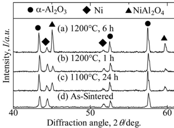
**Fig. 3.** XRD patterns of the sintered Ni/Al<sub>2</sub>O<sub>3</sub> samples with and without heat-treatments.
