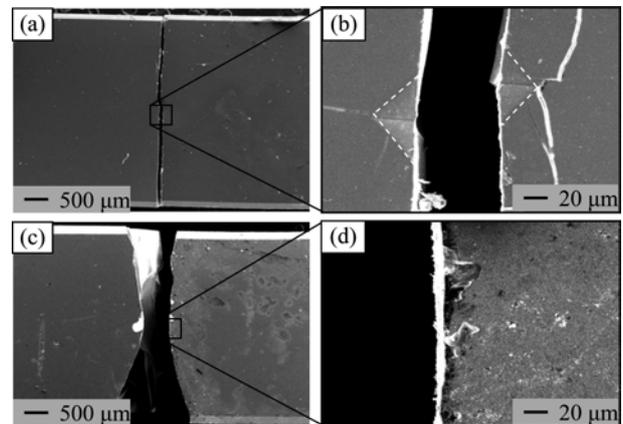
**Fig. 6.** SEM images of bending tested samples; as-cracked (a) and (b), as-healed at 1200 °C for 6 h (c) and (d).
