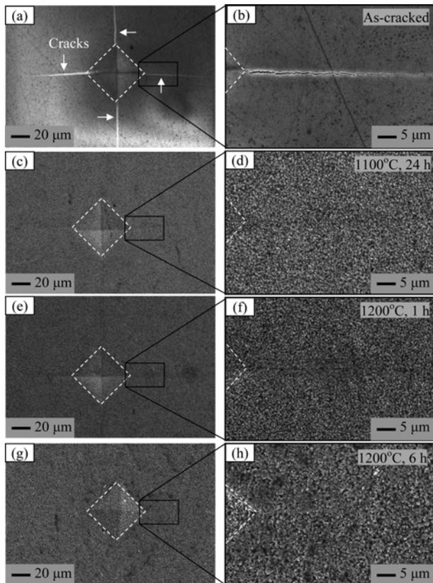
**Fig. 4.** SEM images of surfaces of as-cracked sample (a) and (b), sample heat-treated at 1100 °C for 24 h in air (c) and (d), sample heat-treated at 1200 °C for 1 h in air (e) and (f), sample heat-treated at 1200 °C for 6 h in air (g) and (h).
