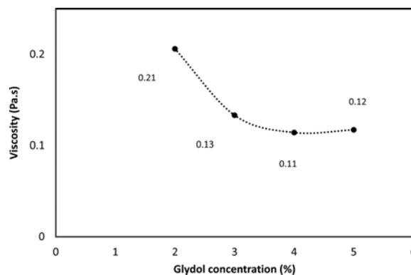
Fig. 1. Viscosity dependence of graphite suspension versus Glydol concentrations.
