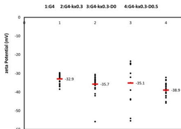
Fig. 5. Zeta potential of 1, 2: graphite suspensions and 3, 4: alumina-zircon-graphite suspensions.
