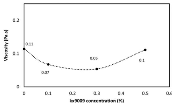
Fig. 2. Viscosity dependence of graphite suspension versus kx9009 concentrations.
