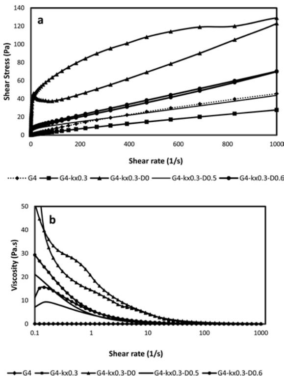
**Fig. 3.** Rheology behavior of suspensions (a) shear stress and (b) viscosity (note that G4 and G4-kx0.3 are graphite suspensions, G4-kx0.3-D0, G4-kx0.3-D0.5, and G4-kx0.3-D0.6) are alumina-zircon-graphite suspensions).
