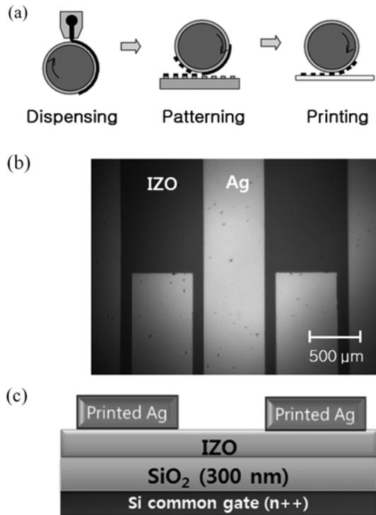
**Fig. 1.** (a) Schematic diagram of ROP process, (b) optical image of the source-drain Ag electrodes fabricated by ROP, and (c) schematic picture of IZO TFTs.
