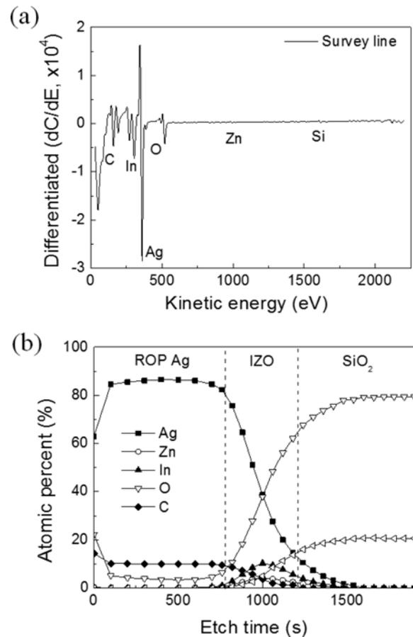
**Fig. 5.** (a) AES survey and (b) depth concentration profile of elements on the Ag/IZO/SiO<sub>2</sub>/Si sample. The sample annealed at 250 °C for 30 min.
