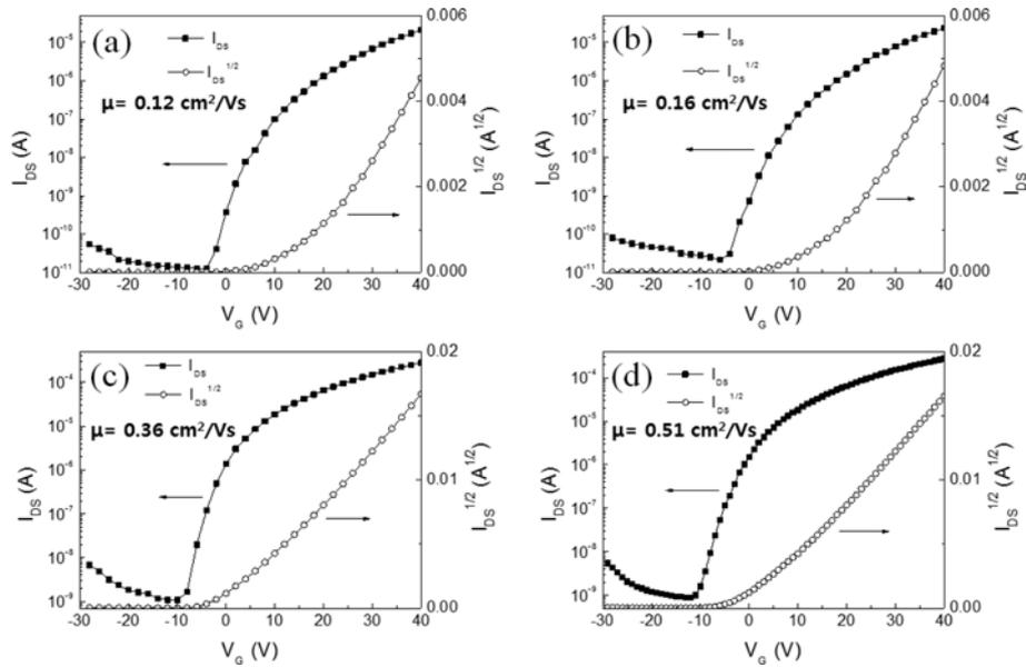
**Fig. 4.** Transfer characteristics of the ROP Ag/IZO TFTs annealed at (a) 120, (b) 150, (c) 220, and (d) 250 °C for 30 min.
