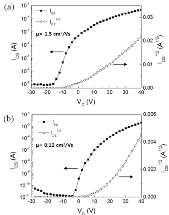
**Fig. 3.** Transfer characteristics of the IZO TFTs with the source-drain electrodes of (a) evaporated Al and (b) ROP Ag.
