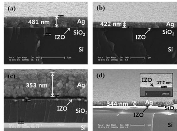
**Fig. 2.** SEM images of Ag/IZO/SiO<sub>2</sub>/Si samples annealed at (a) 120, (b) 150, (c) 220, and (d) 250 °C for 30 min. The inset of Fig. 2(d) is the SEM image of IZO/SiO<sub>2</sub>/Si sample.
