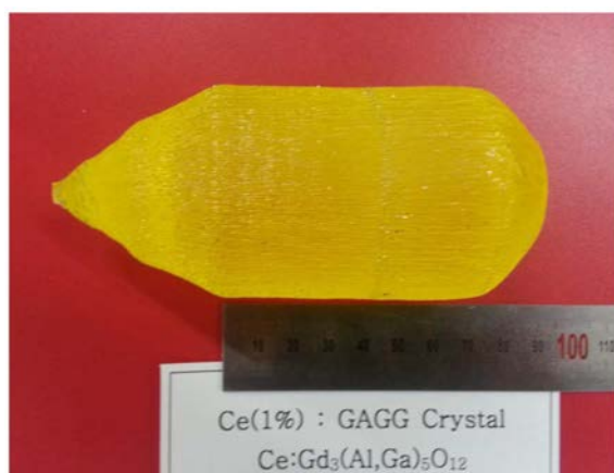
Fig. 1. A GAGG single crystal grown by TPS used in this study.
