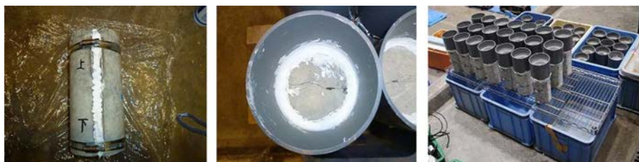
Fig. 2. Specimen preparations for water leakage test.
