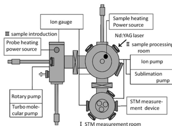
Fig. 1. A schematic drawing of the experimental setup.
