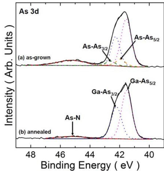
**Fig. 2.** XPS spectra of As 3d photoelectron for (a) as-grown and (b) annealed GaInNAs samples.
