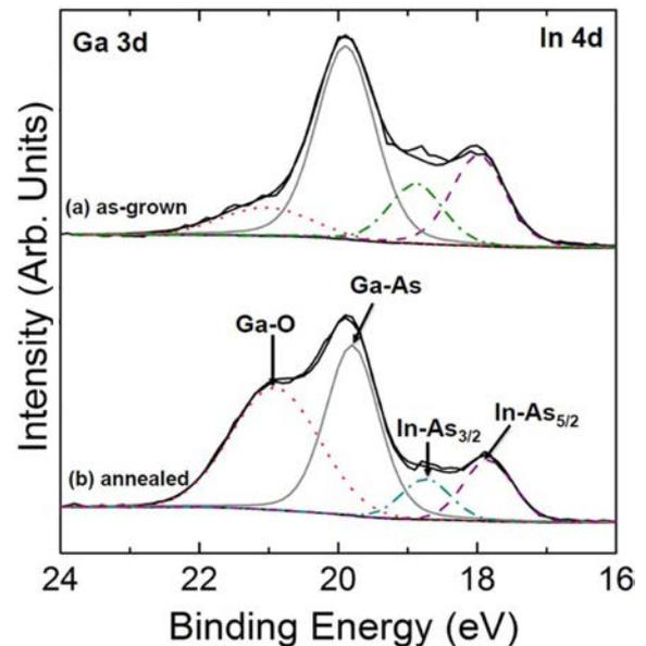
**Fig. 3.** XPS Ga3d/In4d spectrum for (a) as-grown and (b) annealed GaInNAs samples.
