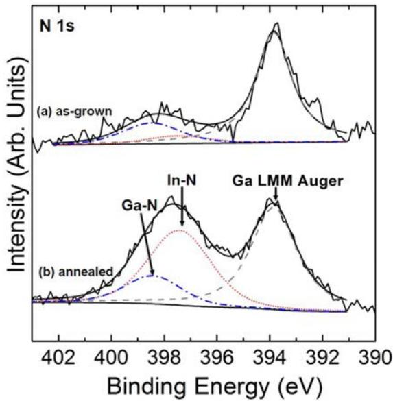
**Fig. 1.** XPS spectra in the N 1s region for (a) as-grown and (b) annealed GaInNAs samples.
