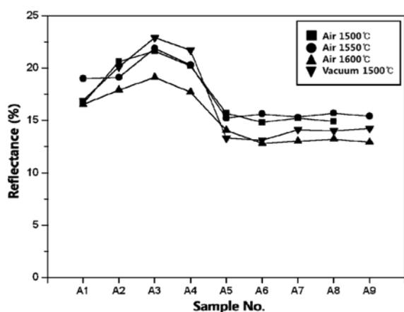
Fig. 1. Reflectivity of black-Al<sub>2</sub>O<sub>3</sub> ceramics according to composition, sintering temperature and atmosphere.
