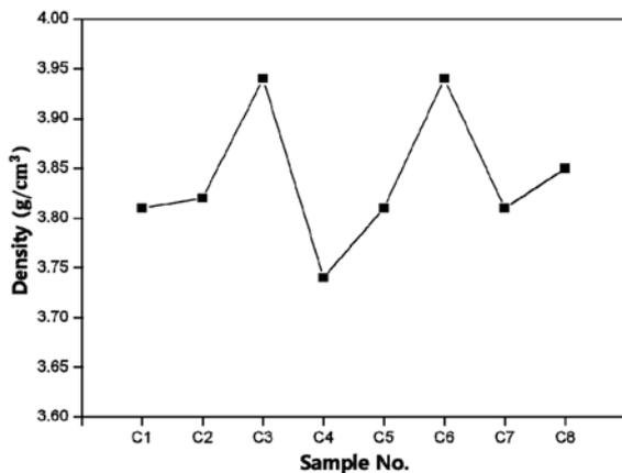
Fig. 4. Sintered density of black-Al<sub>2</sub>O<sub>3</sub> ceramics sintered at 1400 °C for 2 h in air atmosphere according to SiO<sub>2</sub> addition.
