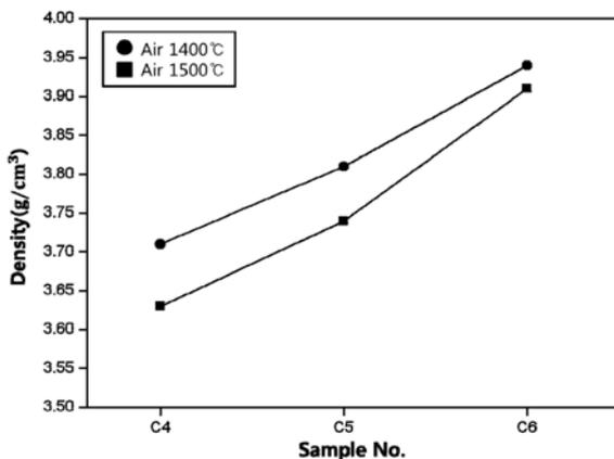
Fig. 5. Sintered density of black-Al<sub>2</sub>O<sub>3</sub> ceramics (C4 ~ C6 samples) sintered at 1400 °C and 1500 °C for 2 h in air atmosphere.
