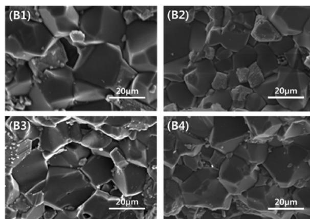
Fig. 3. SEM micrographs of black-Al<sub>2</sub>O<sub>3</sub> ceramics sintered at 1600 °C for 2 h in air atmosphere according to MnO<sub>2</sub> addition.
