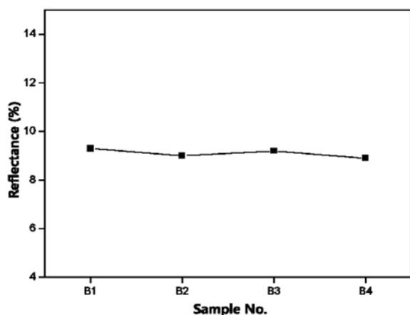
Fig. 2. Reflectivity of black-Al<sub>2</sub>O<sub>3</sub> ceramics sintered at 1600 °C for 2 h according to MnO<sub>2</sub> addition.
