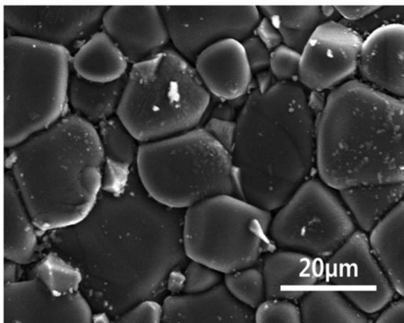
**Fig. 8.** SEM micrograph of black-Al<sub>2</sub>O<sub>3</sub> ceramic (C6 sample) sintered at 1400 °C for 2 h in air atmosphere.
