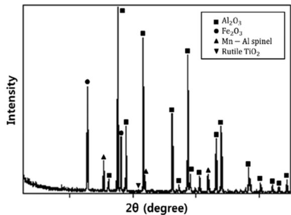
Fig. 7. XRD pattern of black-Al<sub>2</sub>O<sub>3</sub> ceramic (C6 sample) sintered at 1400 °C for 2 h in air atmosphere.
