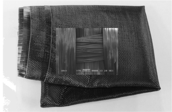
Fig. 1. Photo of woven basalt fibers. SEM micrograph in the center shows the woven pattern.
