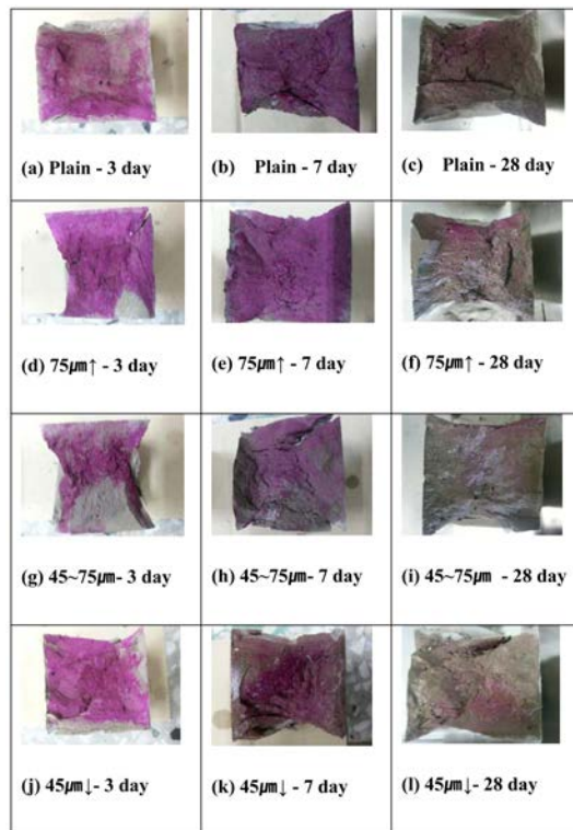
Fig. 3. Carbonation depth of the specimens according to the particle-size separation after carbonation under the supercritical condition.
