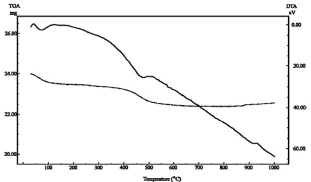
**Fig. 2.** DTA/TG curves of the clay sample.
