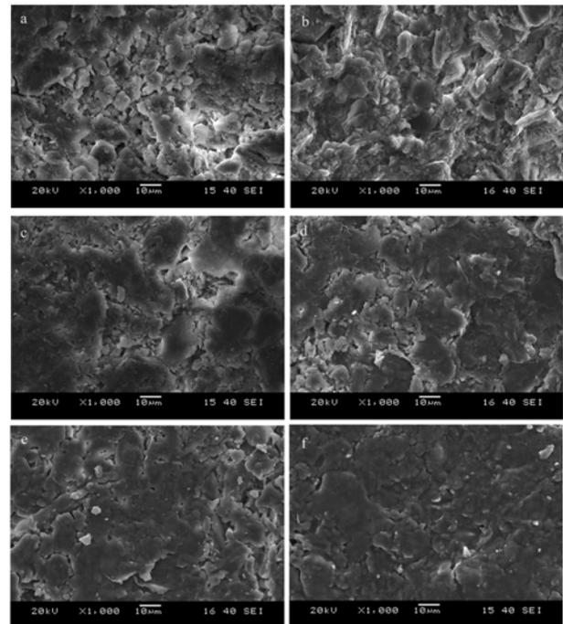
**Fig. 7.** SEM micrographs of the clay samples fired at: (a) 850 °C, (b) 900 °C, (c) 950 °C, (d) 1000 °C, (e) 1100 °C and (f) 1200 °C.
