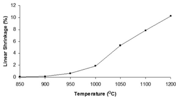
**Fig. 5.** Linear shrinkage values of the KC samples as a function of firing temperature.
