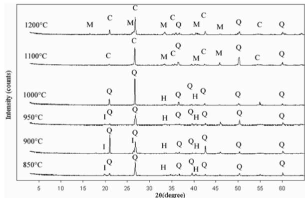
**Fig. 3.** XRD patterns for KC samples fired at different temperatures (Q: Quartz, I: Illite, H: Hematite, M: Mullite, C: Cristobalite).
