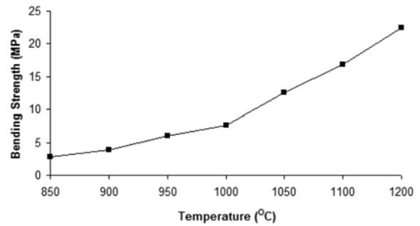
**Fig. 6.** Bending strength values of KC samples fired at different temperatures.
