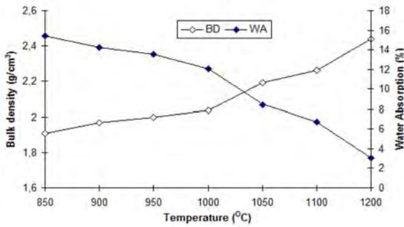
**Fig. 4.** Bulk density and the water absorption values of KC samples fired at different temperatures.
