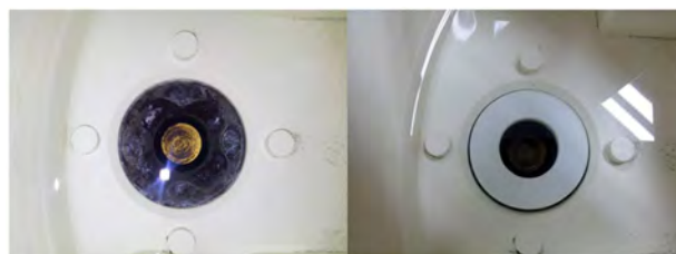
Fig. 7. Standard housing (left-hand-side image) and hydroxyapatite housing (right-hand-side image).
