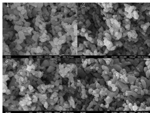
**Fig. 2.** SEM images of Ti-doped HA sintered at 1200 °C for 2 hrs with various addition of titanium; (1) 0.2 wt.%, (2) 0.8 wt.%, (3) 1.6 wt.% and (4) 2.4 wt.%.
