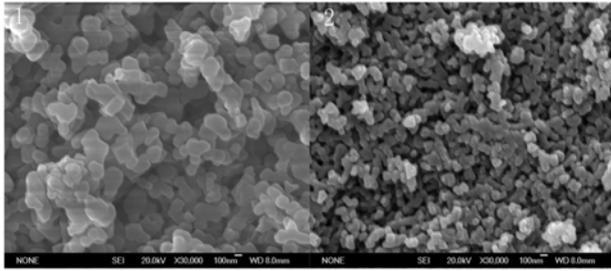
**Fig. 3.** SEM images of HA sintered at 1200 °C for 2 hrs; (1) without the addition of titanium (2) with the addition of 0.8 wt.% titanium.
