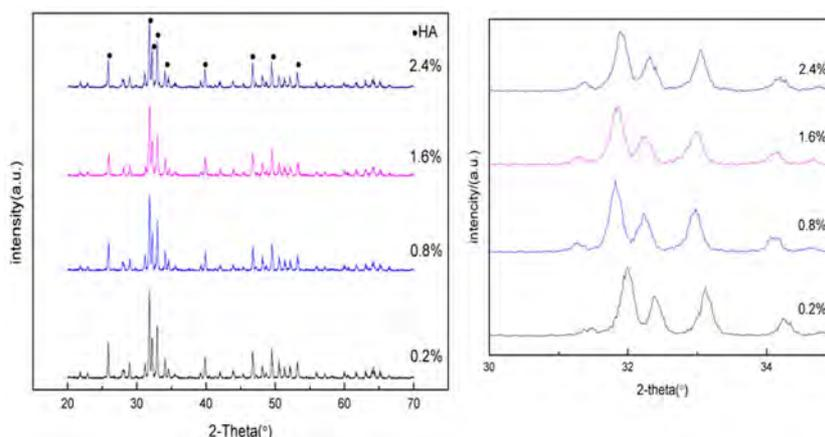
**Fig. 1.** XRD patterns and local magnified patterns of Ti-doped HA sintered at 1200 °C for 2 hrs with various addition of titanium.
