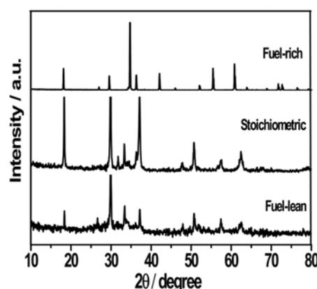
**Fig. 2.** XRD patterns of  $Zn_2SnO_4$  synthesized by a microwave-assisted combustion method.
