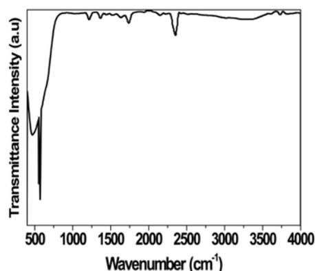
Fig. 5. FTIR spectra of  $Zn_2SnO_4$ .
