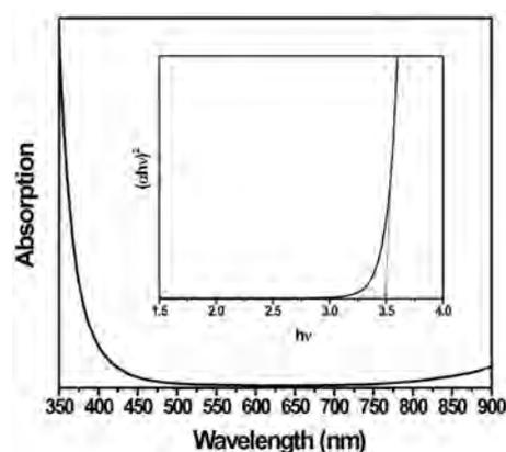
Fig. 6. UV-Vis spectra of  $Zn_2SnO_4$ .
