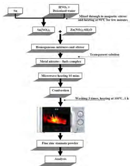
**Fig. 1.** Flowchart for sample preparation of zinc stannate by microwave-assisted combustion method.
