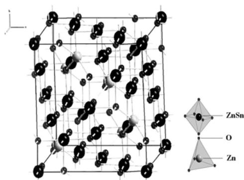
Fig. 3. The results of Rietveld analysis for the rhombohedral structure of  $Zn_2SnO_4$  synthesized using urea as fuel.
