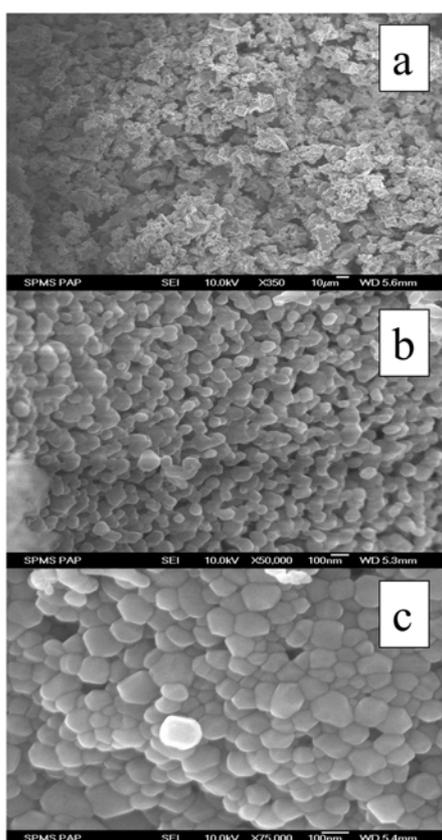
Fig. 4. SEM micrograph of (a) fuel in lean, (b) stoichiometric and (c) rich condition of  $Zn_2SnO_4$  powders.
