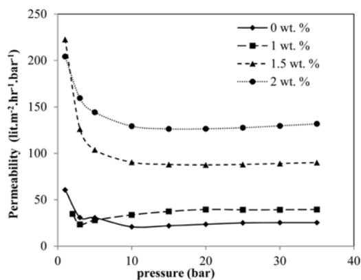
Fig. 7. Permeability of supports versus initial ammonium nitrate content (wt. %).
