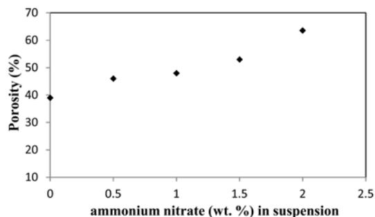
Fig. 3. Dependence of open porosity on initial ammonium nitrate content (wt.%).
