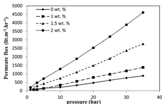
Fig. 6. Permeate flux versus pressure for supports fabricated with different AN contents.
