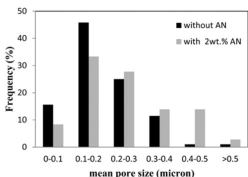
Fig. 5. Pore size distribution of supports surface (a) without and (b) with initial AN (2 wt.%).
