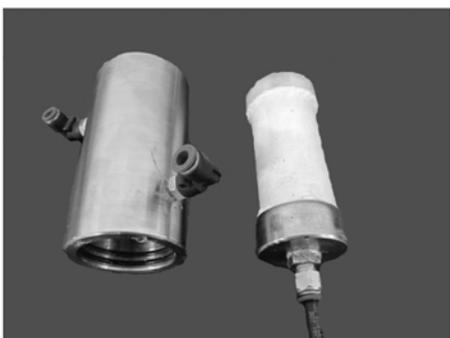
Fig. 2. Module with sealed support.
