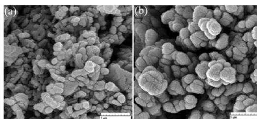
Fig. 4. SEM micrographs of supports' cross section (a) without and (b) with initial AN (2 wt.%).
