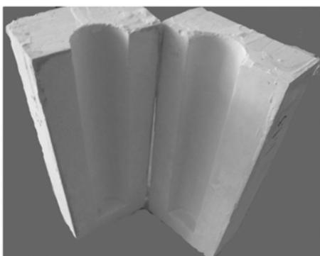
Fig. 1. The photograph of plaster mold.
