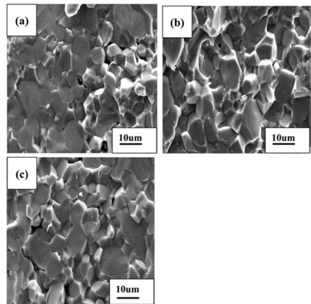
**Fig. 8.** SEM of ceramics under different holding time (a-2 min, b-4 min and c-6 min).
