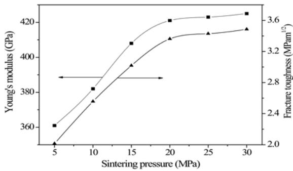
**Fig. 5.** Effect of sintering pressure on Young's modulus and fracture toughness of ceramics.
