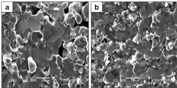
**Fig. 6.** Effect of sintering pressure on microstructure of ceramics (a-5 MPa and b-20 MPa)
