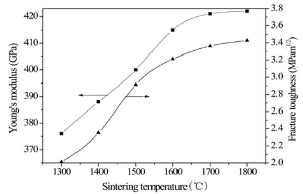
**Fig. 3.** Effect of sintering temperature on Young's modulus and fracture toughness of ceramics.
