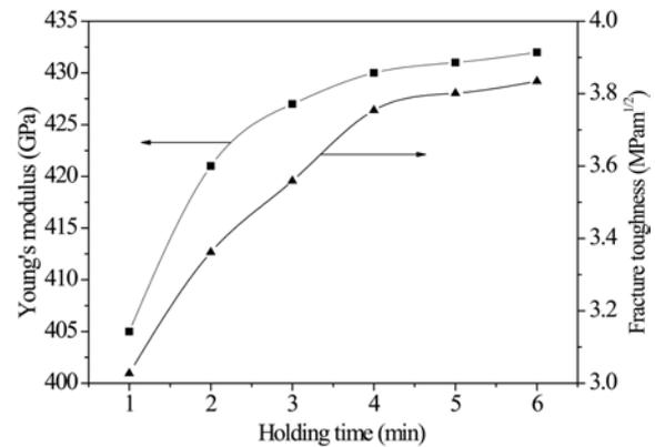
**Fig. 7.** Effect of holding time on Young's modulus and fracture toughness of ceramics
