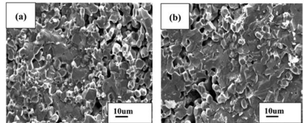
**Fig. 4.** SEM of ceramics under different sintering temperature (a-1500 °C and b-1700 °C).
