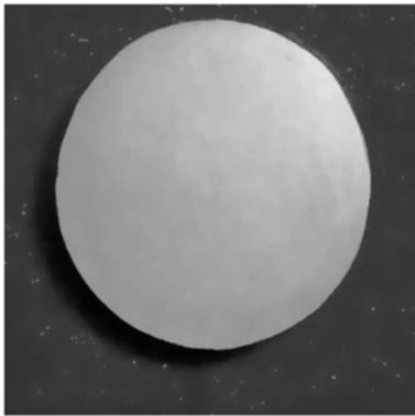
**Fig. 2.** Picture of YAG/ZrB<sub>2</sub> ceramics sample.
