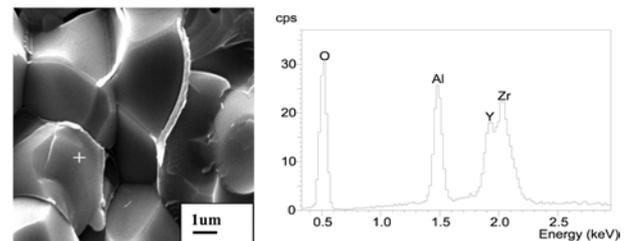
**Fig. 9.** SEM and EDS of ceramics sintered under 1700 °C, 4 min and 20 MPa.
