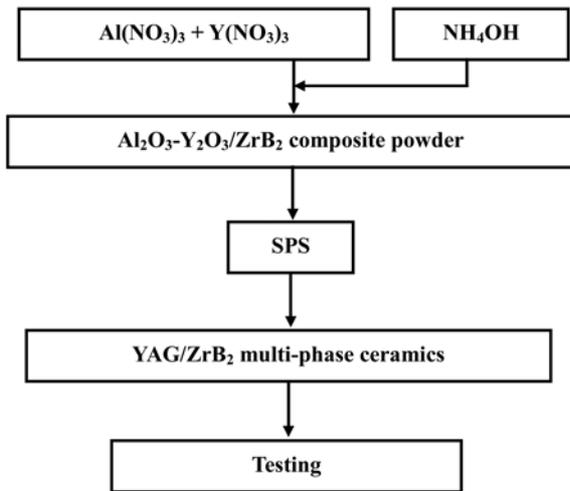
**Fig. 1.** The process flow diagram for preparing YAG/ZrB<sub>2</sub> ceramics.
