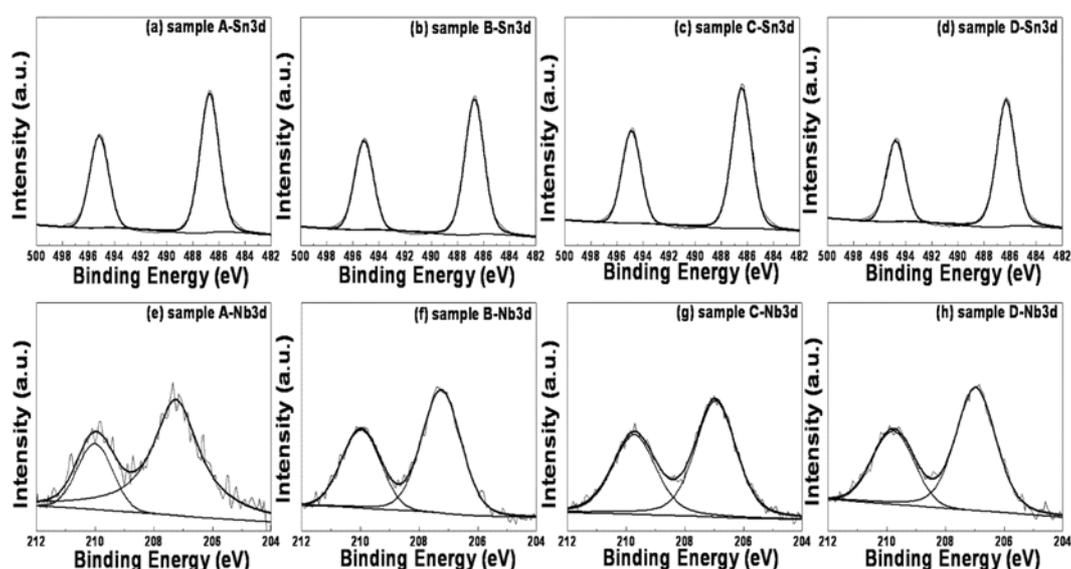
Fig. 2. XPS spectra of the Sn 3d and the Nb 3d core levels obtained from samples A, B, C, and D.
