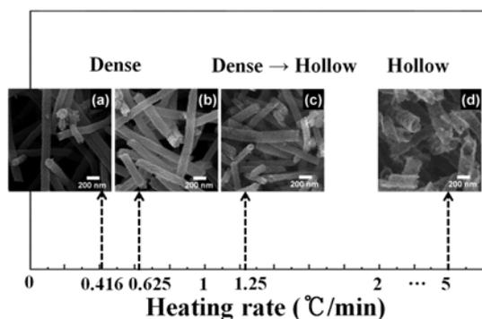
**Fig. 5.** dependence of heating rates ( $^{\circ}\text{C}/\text{min}$ ) of sample D; (a) 0.416, (b) 0.625, (c) 1.25, and (d)  $5^{\circ}\text{C}/\text{min}$  during calcination at  $500^{\circ}\text{C}$ .
