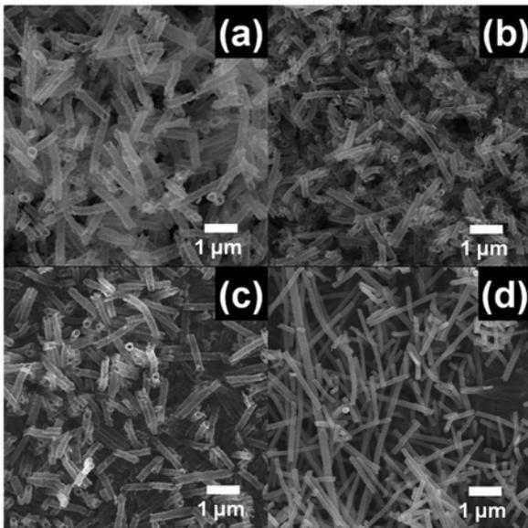
**Fig. 3.** FE-SEM images obtained from (a) sample A, (b) sample B, (c) sample C, and (d) sample D after calcination at 500 °C.
