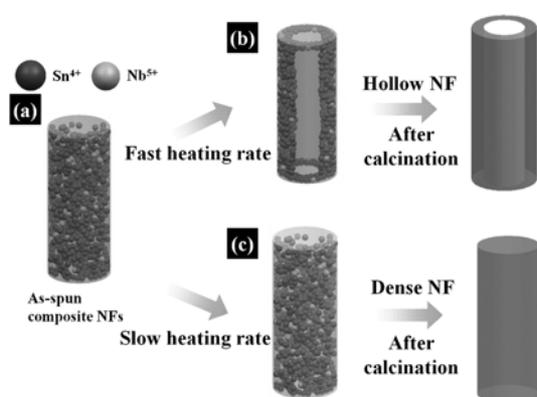
**Fig. 6.** A schematic diagram on the formation process of hollow and dense Nb-doped  $\text{SnO}_2$  NFs depending on the heating rates.
