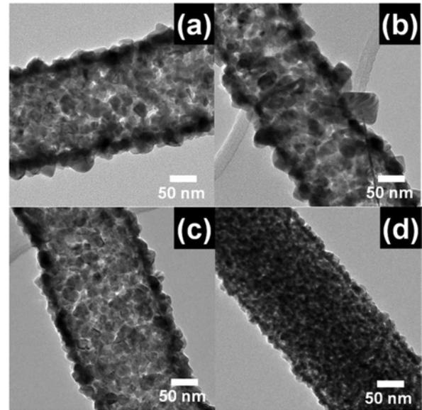
**Fig. 4.** TEM bright field images obtained from (a) sample A, (b) sample B, (c) sample C, and (d) sample D after calcination at 500 °C.
