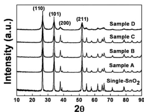
Fig. 1. Powder XRD data of single SnO<sub>2</sub>, and of samples A, B, C, and D obtained after calcination at 500 °C.
