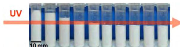
**Fig. 3.** Demonstration of the sedimentation rate measurement.
