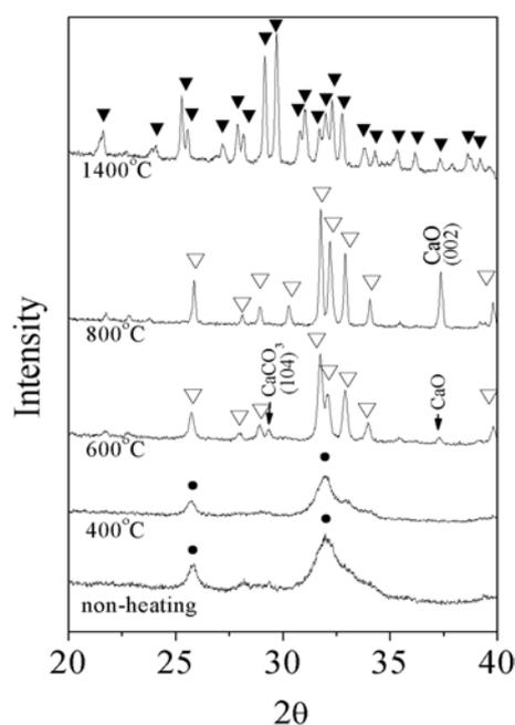
**Fig. 1.** Variation in XRD patterns at different heating temperatures. ● : apatite; ▽ : HA; ▼ : TTCP.
