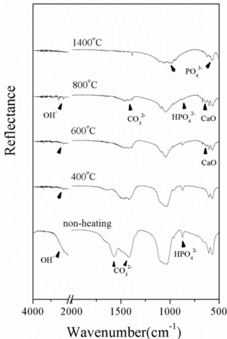
Fig. 5. FTIR absorption spectra of different heating temperatures.
