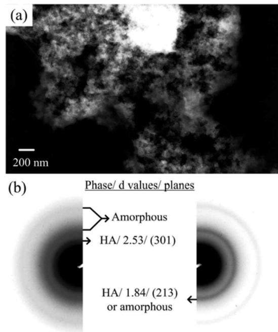
**Fig. 4.** Bright field (BF) image of precipitates mixed with carbon black (a) and respective SAD patterns with indices (b).
