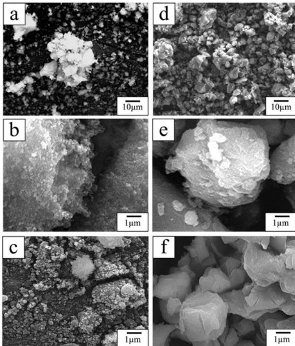
**Fig. 3.** Variation in morphologies of precipitates mixed with carbon black (a), (b) and (c); after 1400 °C sintering temperature of (d), (e) and (f). (b), (e): non-dispersed; (c), (f): dispersed powders.
