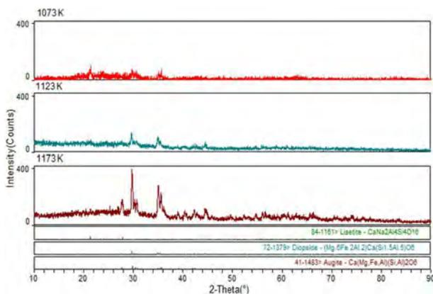
**Fig. 4.** XRD patterns of glass ceramics produced from fly ash treated at (a) 1073 K, (b) 1123 K and (c) 1173 K for 120 minutes.
