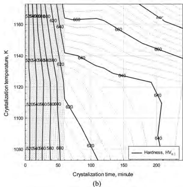
**Fig. 5.** (a) Hardness curves as a function of crystallization time and temperature, (b) Iso-hardness diagrams.
