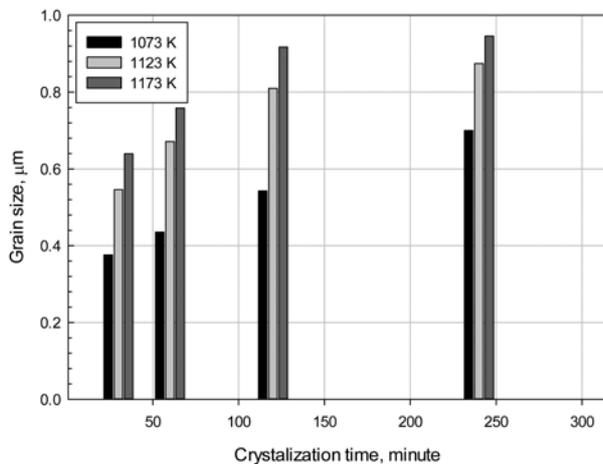
**Fig. 3.** Variation of grain size of the glass-ceramics produced from fly ash depending on the crystallization time and temperature.
