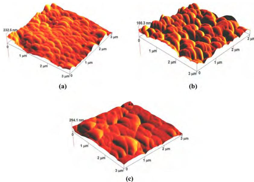
**Fig. 2.** AFM images of glass ceramics produced from fly ash heat treated at (a) 1073 K, (b) 1123 K and (c) 1173 K for 120 minutes.
