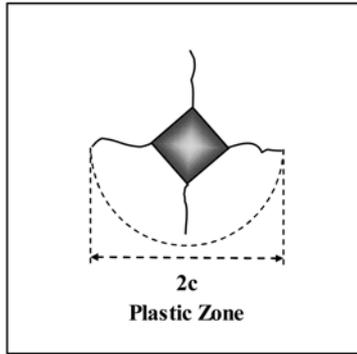
**Fig. 1.** Schematic view of the indentation mark and crack length.
