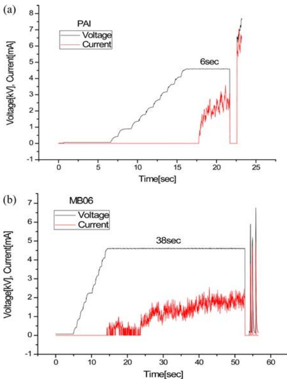
Fig. 8. The V-t properties of PAI-CS hybrid films. (a) PAI and (b) MB06.
