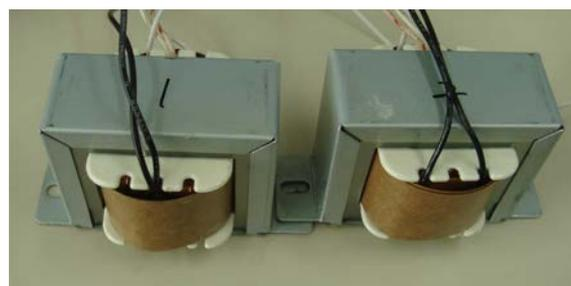
Fig. 2. TR modules for temperature rising test.
