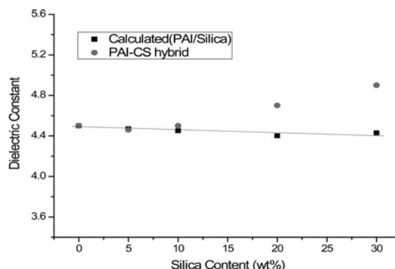
Fig. 7. The dielectric constant with silica content in PAI-Si hybrid film.
