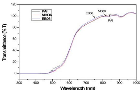
Fig. 4. The effect of silica on the UV-Vis spectra of PAI-CS hybrid films.
