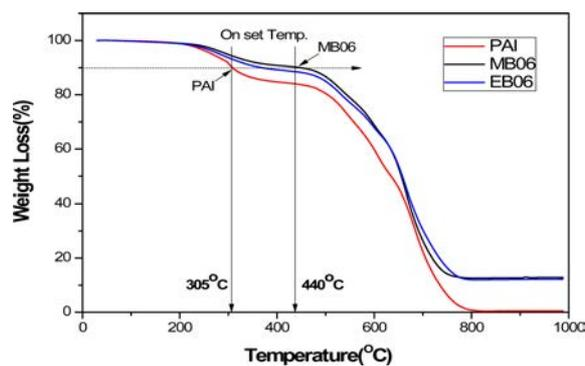
Fig. 6. The TGA curves of PAI-CS hybrid films.
