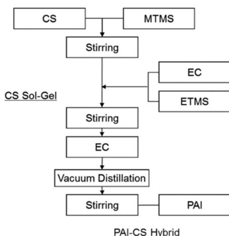
Fig. 1. The preparation of PAI-CS hybrid.
