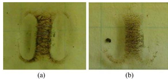
Fig. 10. The surface photography after tracking erosion. (a) PAI and (b) MB06.
