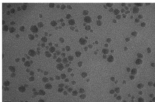
Fig. 5. The TEM photograph of PAI-CS hybrid (MB06).
