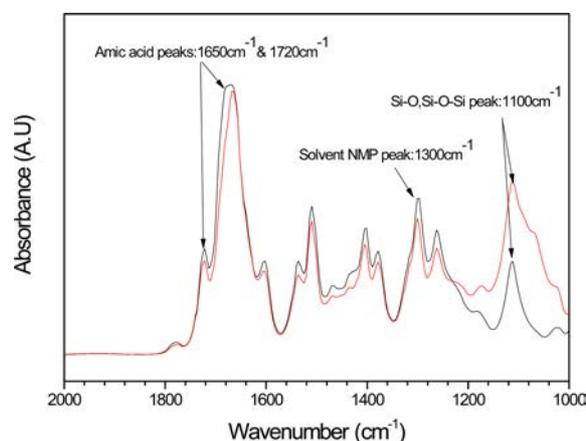
Fig. 3. FT-IR spectra of the PAI-CS hybrids with and without silica.
